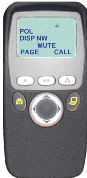
*The scan feature allows you to monitor traffic on different channels by scanning a preprogrammed list of channels. Your radio can have several different scan lists. These lists must be enabled by a qualified radio technician.*
