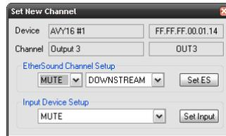
On top of window presents current device output assignment.
