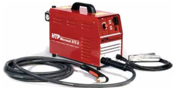
Just feed it 220 volts of power and clean compressed air, and it will easily blast through ¾" solid steel plate at 7 ½"/min and severance cut 1 ⅛" steel. The arc is ignited without high frequency, extending consumable life while at the same time eliminating any interference with computers, TVs or telephones. And it features automatic arc re-ignition for cutting expanded metal.
