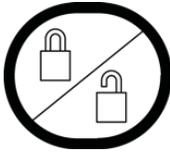
This is the **LOCK/RELEASE** key. It is used to lock and unlock the display. If the HOLD feature was enabled during setup and calibration, pressing this key (after obtaining a stable weight) will cause the indicator to lock onto the weight. Pressing this key again will unlock the display and return it to zero.
