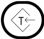
This is the **TARE** key. It is a dual function key. Pressing it and pressing the **PRINT/ENTER** key (Pushbutton Tare mode) will cause the current gross weight to be stored as the new tare weight and change the weight display to the net weight display mode (Net annunciator will turn on). Pressing this key, entering a numeric value (Keypad Tare) and then pressing the **PRINT/ENTER** key will cause the value entered to be accepted as the new tare weight.
