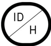
This is the **ID/HEIGHT** key. This key is used to display and enter an identification (ID) number use in the ID Storage feature and to enter the height (feet and inches or centimeters) for the Body Mass Index (BMI) calculation.
