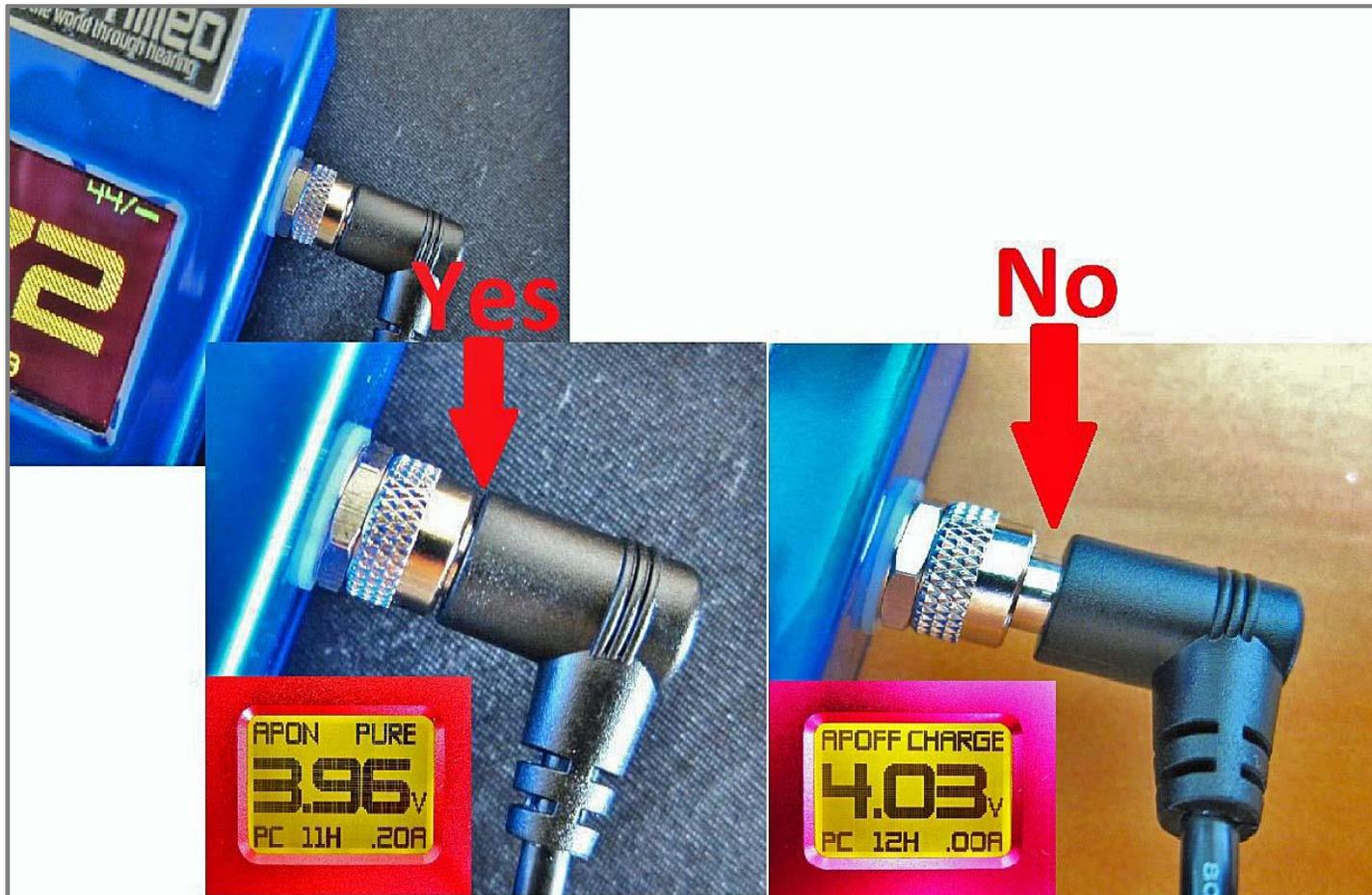
Figure 3 Insert the power cable into the Audiophileo, then **GENTLY** screw it on, then push it fully in. **Note that with newer units it is only necessary to gently thread the cable in. After that it is already fully pushed in.**
