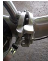
Lift up lever to release pin from frame
