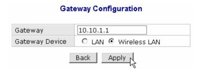
**5)** Select 'Wireless LAN' and input 'Gateway address'. It must be same as the ones registered at the Wireless Router (Access Point). And click 'Apply' button.
