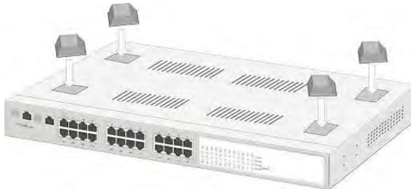
Attaching Rubber Feet to each corner on the bottom of the Switch
