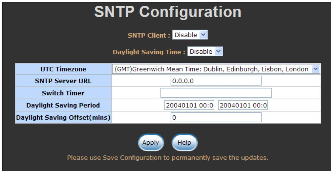
The screenshot shows the SNTP Configuration interface. At the top, it says "SNTP Client : Disable" and "Daylight Saving Time : Disable". Below this is a table with the following fields:
