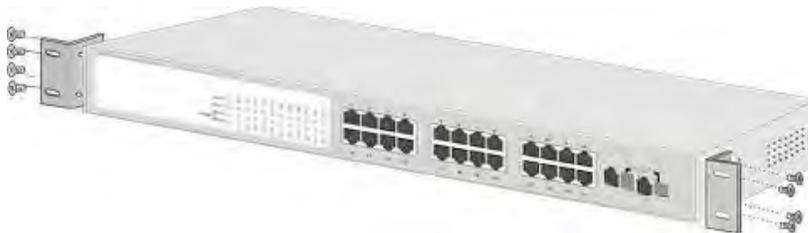
Attach mounting brackets with screws
