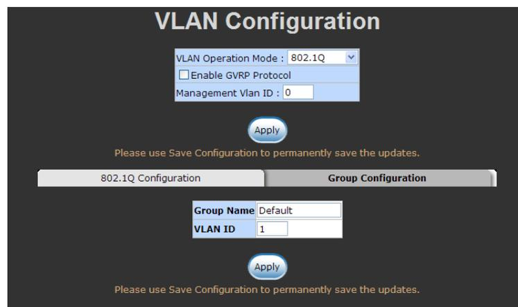
This screenshot is similar to the previous one but shows the configuration fields for the selected group. The 'Group Name' field contains 'Default' and the 'VLAN ID' field contains '1'. There is an 'Apply' button below these fields. The rest of the interface, including the top settings and the '802.1Q Configuration' tab, remains the same.
