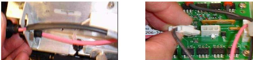
**Figure 9** Connecting the HV PCA to the chassis.
