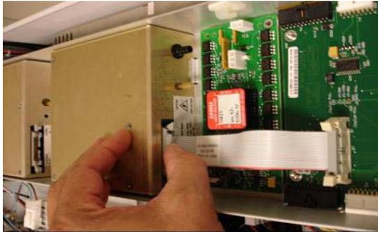
**Figure 5** Connecting the valve PCA to the Vcap/Vchamber power supply.
