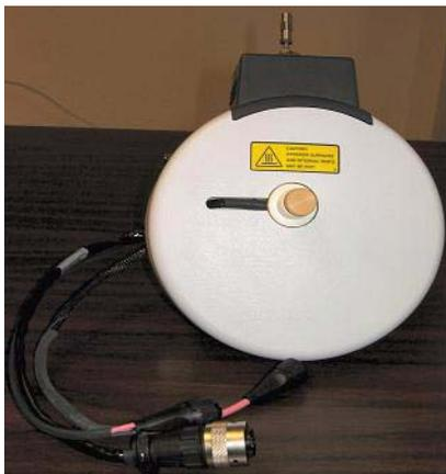
Figure 15 Multimode Spray Chamber
