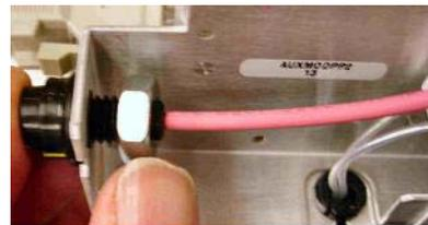
**Figure 8** Connecting the APCI HV to the chassis.
