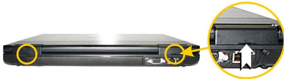
4. Open the lid of the mobile thin client. Using the plastic alignment tool or your finger nails, carefully pry off the switch cover starting at the corners as indicated in Figure 6.
