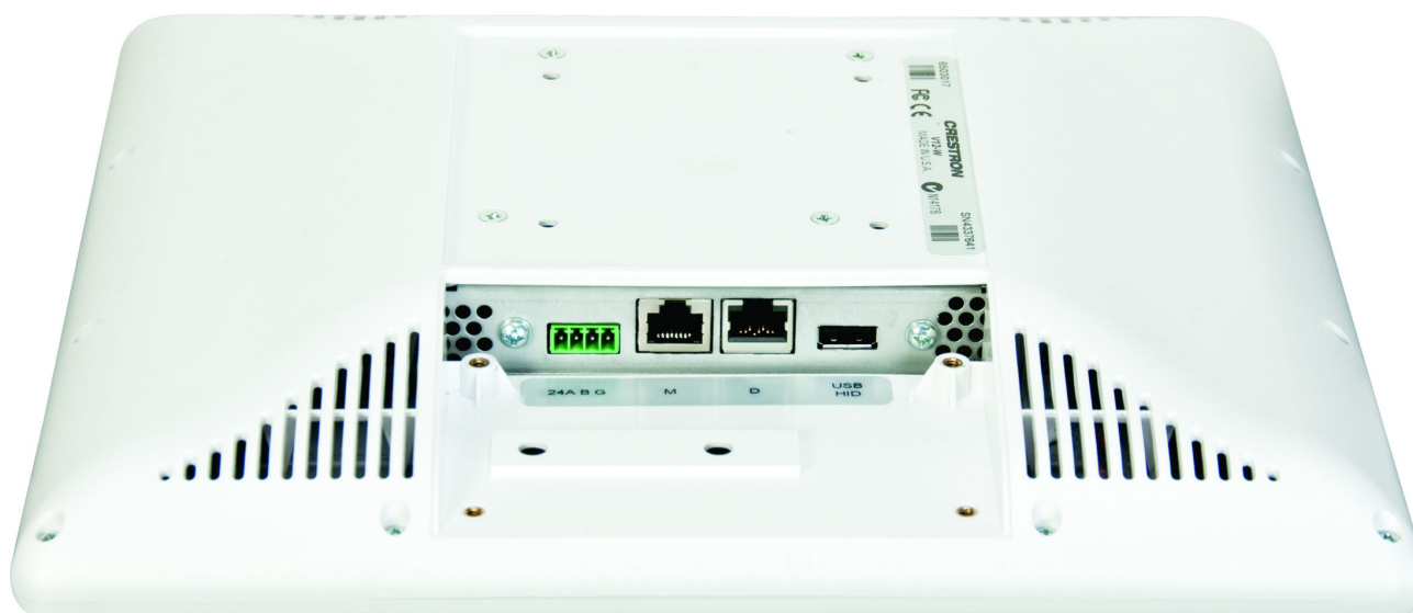
V-Panel Physical View (Rear Showing Connector Ports)
