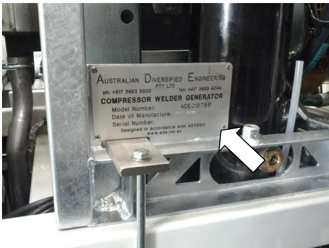
ID plate affixed near the oil separator tank
