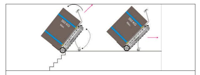
• Drive the stairrobot over the top and keep the stairrobot balanced until the folding wheel locks into position; resume the forward movement
