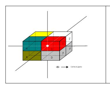
Before positioning the load on the platform the centre of gravity of the load has to be determined
