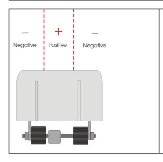
The centre of gravity of the load should be within the positive area between the tracks.
