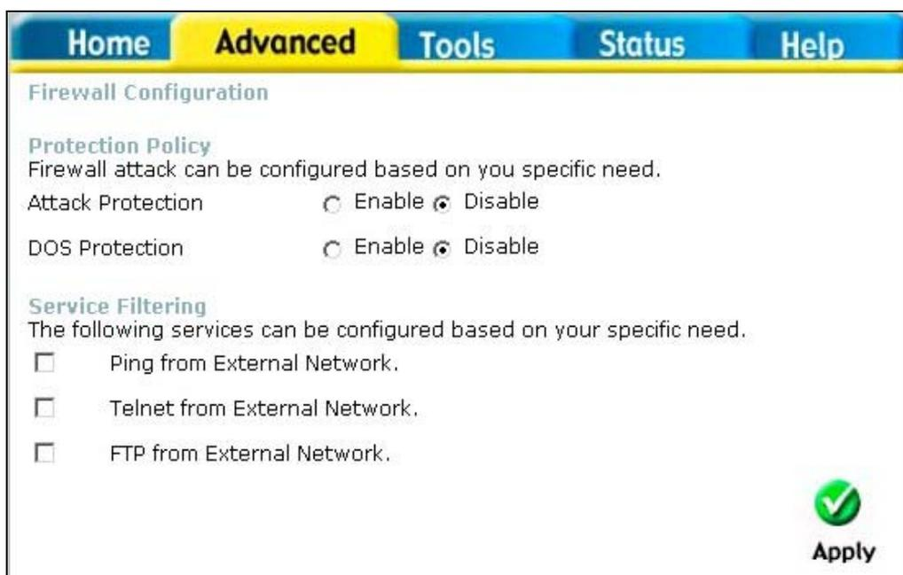
Figure 4- 5. Firewall Configuration Menu
