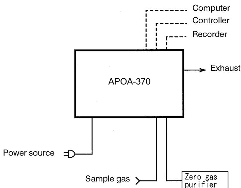
**Fig. 1 System configuration**
