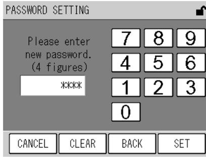
**Fig. 81 PASSWORD SETTING screen (requiring a new password)**
