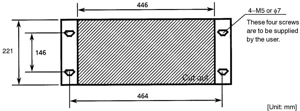
**Fig. 105 Mounting the APOA-370 on a panel**
