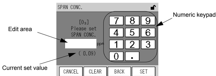
Fig. 16 A screen for value setting (SPAN CONC.)
