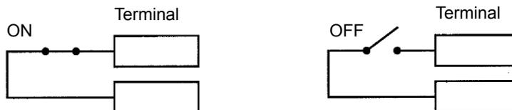
Fig. 103 ON/OFF status of a contact terminal
