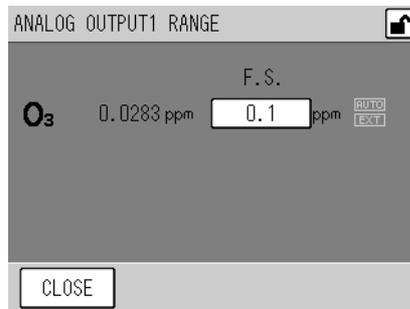
**Fig. 66 ANALOG OUTPUT RANGE screen (ANALOG OUTPUT1)**
