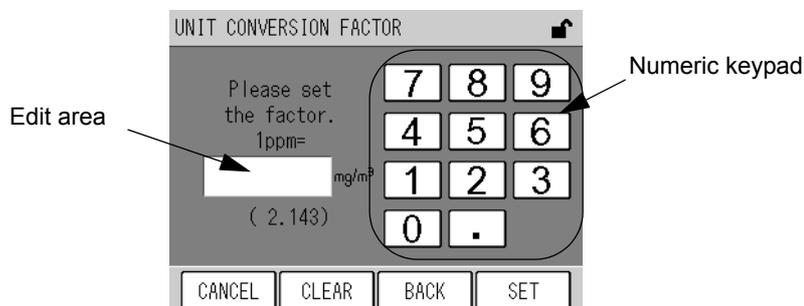
**Fig. 74 UNIT CONVERSION FACTOR screen for setting**
