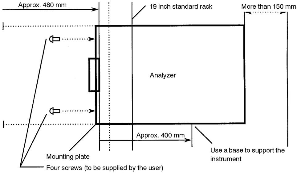
**Fig. 104 Mounting the APOA-370 on a 19-inch rack**
