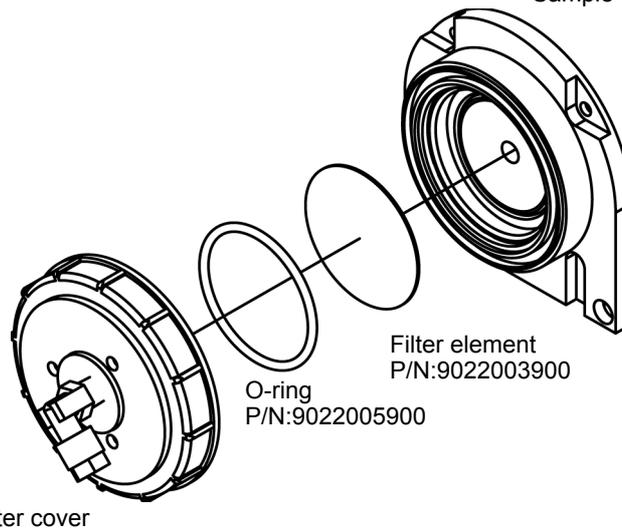
**Fig. 99 Exploded view of filter element**
