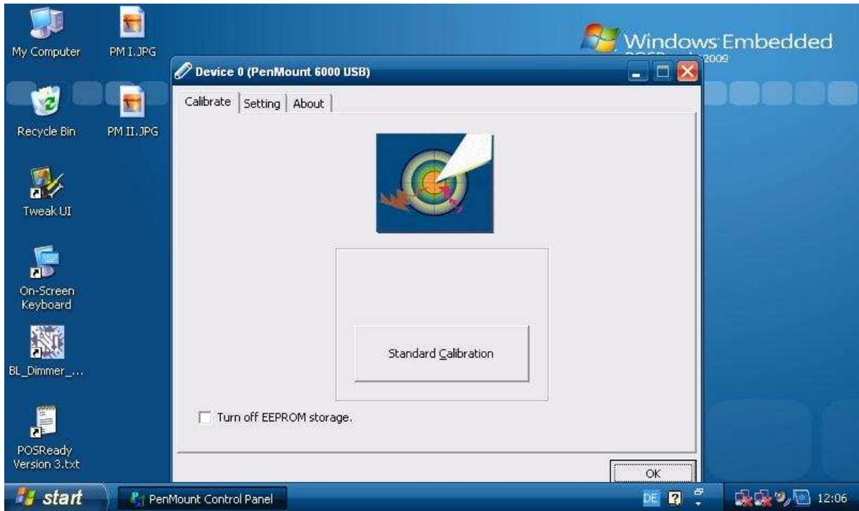
4. Pressing the [Standard Calibration] button on the main window activates the calibration screen to carry out calibration of the Touch Panel. Briefly touch the centre of the red square splayed on the screen in order as they appear. Once calibration is carried out, the calibrated value is saved. Since the calibrated value is read from the setting file at the time of the next start up, there is no need to carry out calibration again.
