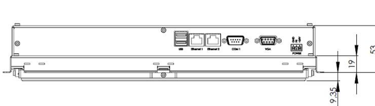
Picture 26: dimensions front frame for **Touch-it XPC 15"**
