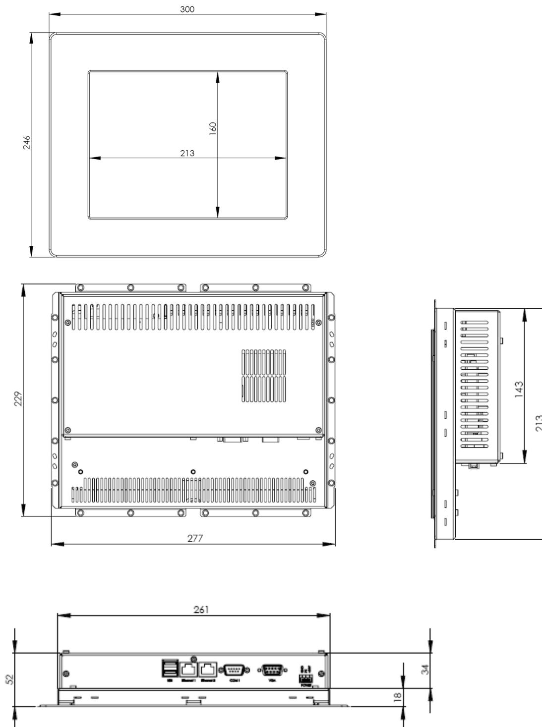
Picture 23: dimensions front frame for **Touch-it XPC 10,4"**
