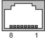
Picture 13: pin assignment Ethernet (RJ45 socket)
