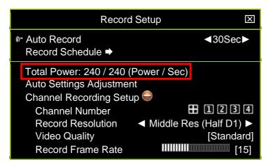
To distribute the recording power into four channels by click the total power (as upper red border).
