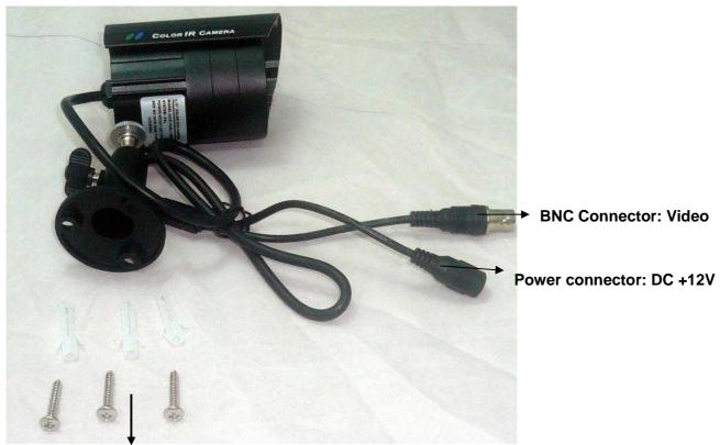
Cap and screws for wall-mount installation
