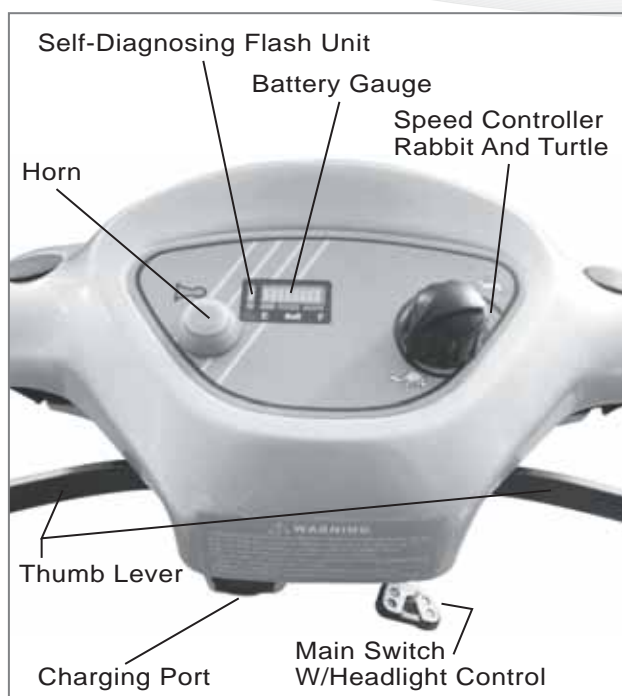
Figure 2 - HS-580 Control Panel
