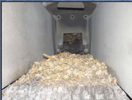
Large wood chips w/turkey manure (ready for firing)
