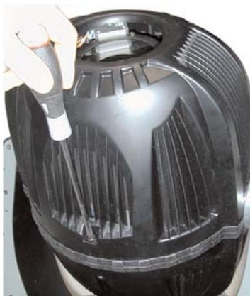
Remove the housings to expose the projector's internals.
