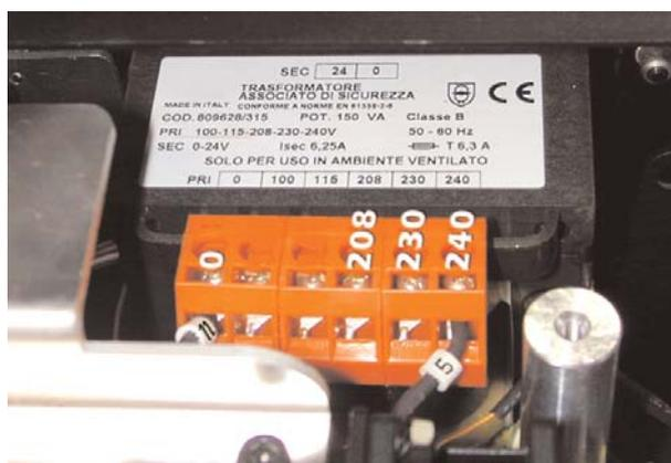
Select a voltage from amongst 208, 230 or 240V by disconnecting cable n° 5 and moving it to the correct voltage. Refer to the sticker located on the transformer to ensure the proper terminal is selected for your requirements.
