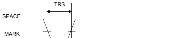
Figure 2.1.1 Minimum Reset Pulse Width (pin 6)
