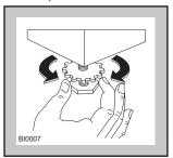
Accurate levelling prevents vibration, noise and displacement of the machine during operation. Never place cardboard, wood or similar materials under the machine to compensate for any unevenness in the floor. After having
