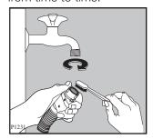
Turn off the water tap. Unscrew the water inlet hose. Clean the filter using a hard bristle brush. Tighten up the inlet hose.
