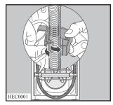
3. With the supplied spanner unscrew and remove the central rear bolt A. Slide out the relevant plastic spacer.
