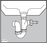
Push the drain hose onto the spigot and secure with a clip, ensure a loop is formed in the drain hose (see diagram) to prevent waste from the sink entering the washing machine.
