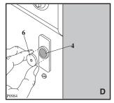
If the door has to be opened from left to right, invert the position of the plates (7), the magnet (4) and the plate (5) (Fig. B and E). Mount the counter-magnet (6) and the hinges (1) as previously described.
