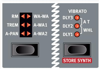
Selector buttons are used to select one setting in an array. They have a set of round or triangular LEDs to indicate the current setting. Press the button several times to cycle through the possible options.
