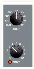
*Hold Shift and turn a knob to view the stored setting of a parameter in the display, without changing it.*
