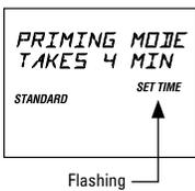
After the initial software indicators are shown, this display will appear. This display is indicating that the system is in **PUMP PRIMING MODE**. This mode will last for 4 to 5 minutes before automatically exiting and entering the normal operation mode. You can also manually exit the **PUMP PRIMING MODE** after the pumps are primed.
