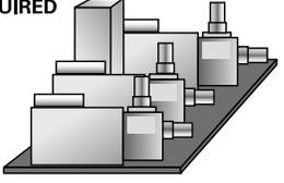
REMOTE ABOVE-GRADE EQUIPMENT, max. 20 ft. pipe run from swim jets with minimal elbows/fittings (Rainproof vented enclosure and optional remote upgrade kit required)
