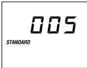
At initial power-up, this display will appear, and the system will show 4 sets of numbers in succession (ie. 100 then 114 then 28 then 240). These numbers represent the current software revision, and the system input voltage.
