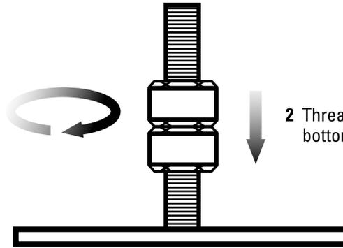
2 Thread two hex nuts down to within 2.5 cm (1 in.) of bottom of foot plate
