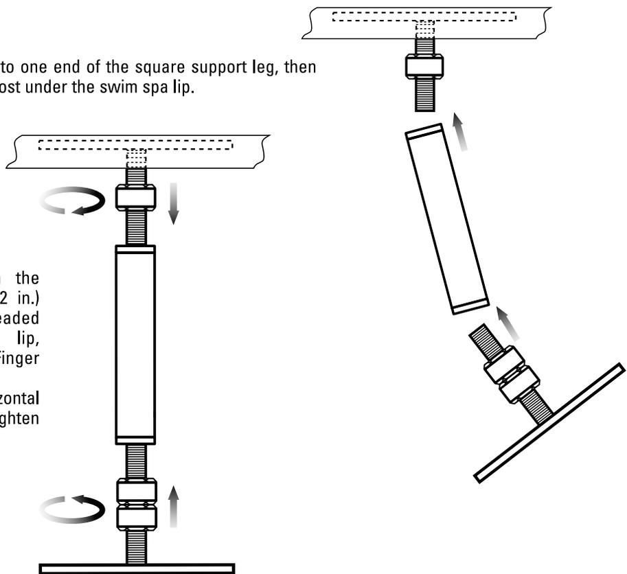
4 Bring the two hex nuts on the foot plate up about 5.1 cm (2 in.) and the hex nut on the threaded post under the swim spa lip, down about 5.1 cm (2 in.). Finger tighten until the leg is secure. Loosen the hex nuts on the horizontal rod so that the leg is level and tighten until the leg is secure.
