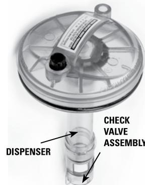
Expose the large Refill hole at the end of the tube and add 5 or 6 tablets. Do not overfill dispenser as performance will be affected. Turn to expose the most number of smaller holes and allow water to circulate for 3 to 4 hours before testing level. Adjust to lesser number of holes as necessary to maintain a level of 2-4 PPM Sanitizer.
