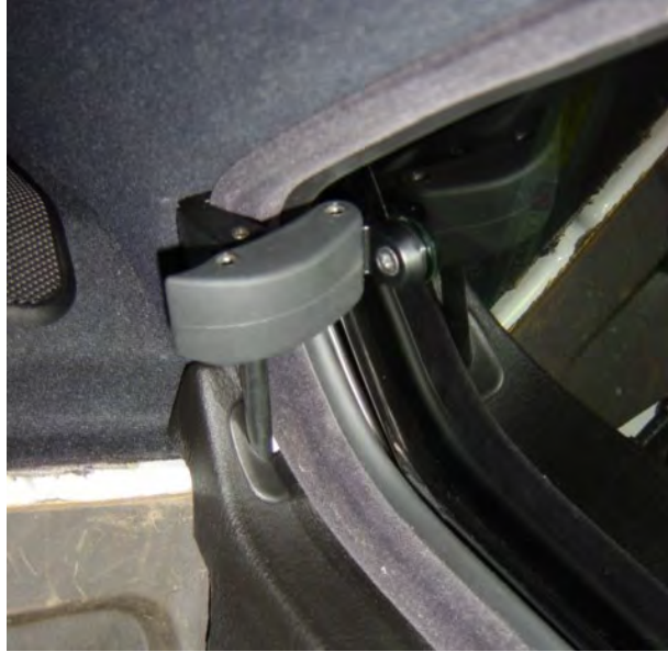
Figure 41 – Rear Panel Trim Piece Installed
