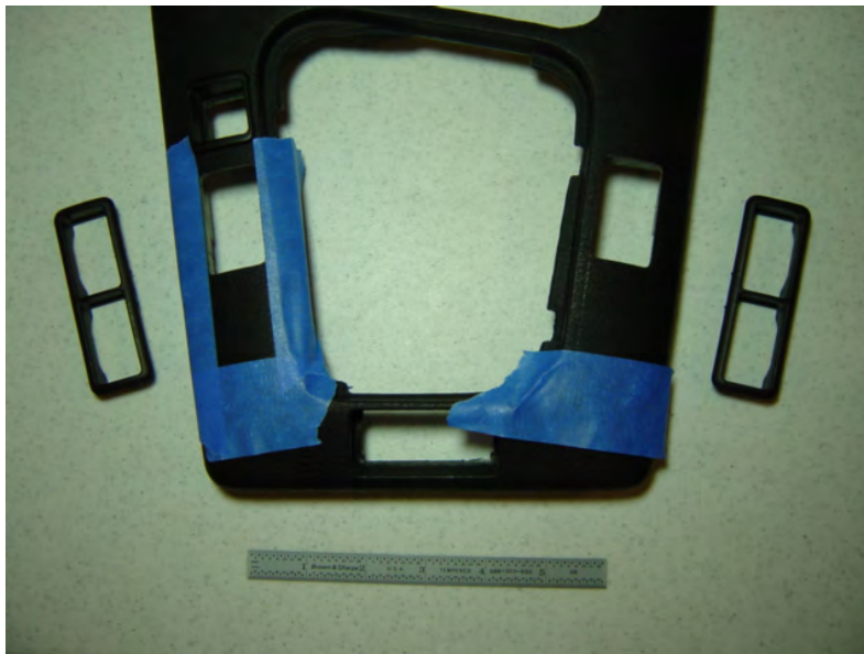
Figure 30 – Cutout Area Marked and Taped
