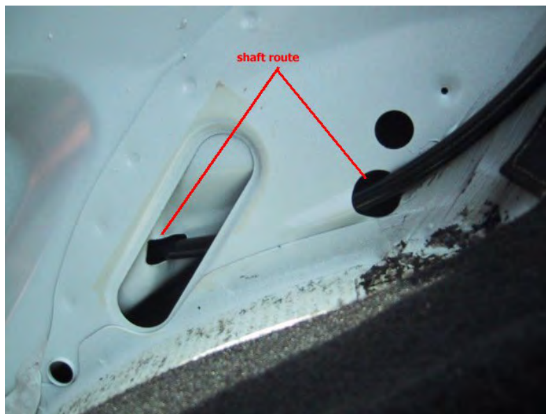
Figure 36 – Routing Flex Shaft toward Window Motor (Picture courtesy D. Ortiz)
