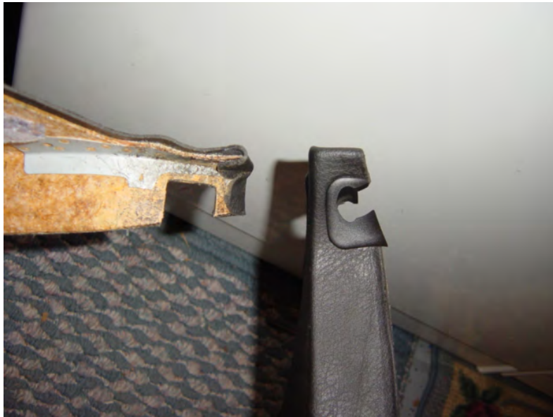
Figure 39 – Rear Panel Cut for Trim Pieces
