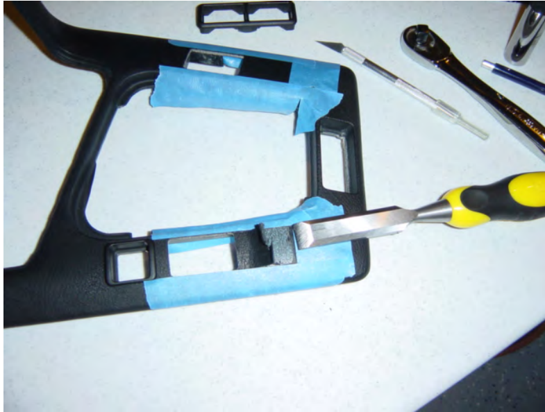
Figure 31 – Removing Black Vinyl Covering on Shifter Console
