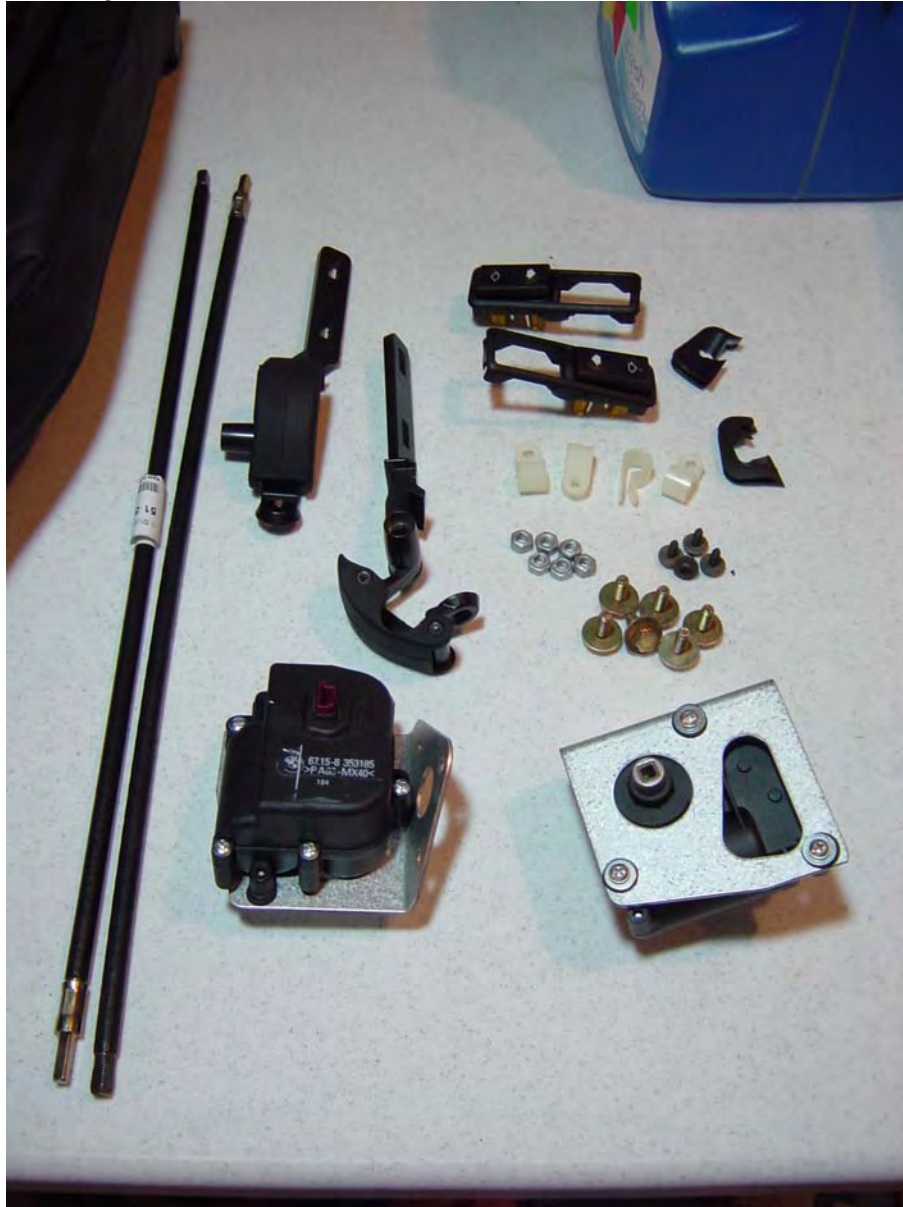
Figure 1 - Electric Hinged Window Kit and Lt/Rt Rear Panel Trim Pieces (top right)
