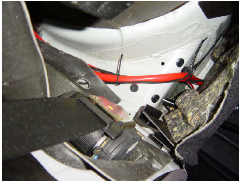
Figure 35 – Routing supplemental harness connector (O shown) under carpet
