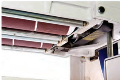
Smooth multi groove Poly-V drive belt
