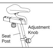
post upward or downward, release the adjustment knob into an adjustment hole in the seat post, and firmly tighten the adjustment knob. **Make sure that the adjustment knob is engaged in an adjustment hole.**
