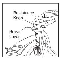
downward. The flywheel should quickly come to a complete stop.
