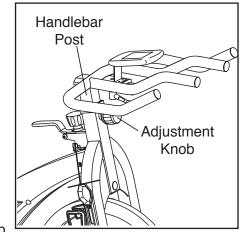
into an adjustment hole in the handlebar post, and firmly tighten the adjustment knob.
