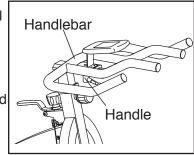
Note: The handle functions like a ratchet. To loosen the handle, turn the handle counterclockwise, pull the handle outward, turn the handle clockwise, push the handle inward, and then turn the handle counterclockwise again. Reverse this process to tighten the handle installed in accordance with all local codes and ordinances.
