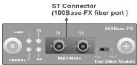
Figure 3-2. 100FX module with SC connector
