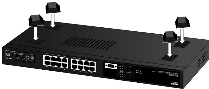
Figure 2-4. Attaching Rubber Feet to each corner on the bottom of the switch
