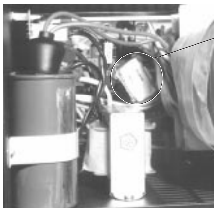
120 VAC Jumper (cable-tied to wire harness)
