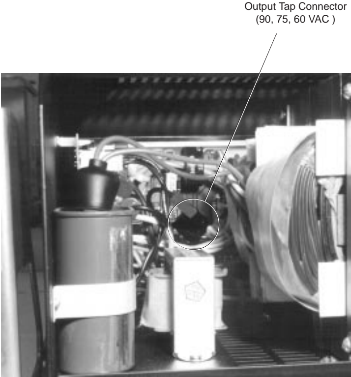
Output Voltage Configuration Taps (from ferroresonant transformer)
