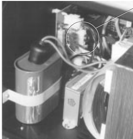
240 VAC Jumper (connected to backplane board)
