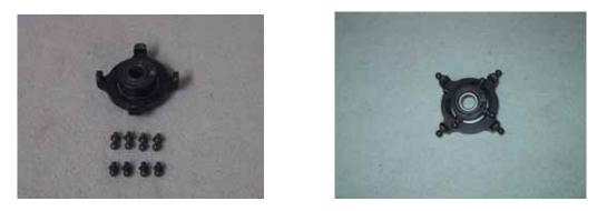
The swashplate is next; install 4 ea medium balls on the inner ring, using loctite. After installing these balls, make sure the eyeball in the center of the swashplate moves freely. If not, check that the threads of the balls haven't gone in too deep, pushing on the eyeball. Remove some of the threaded end, if necessary. 4 ea short balls go in the outer ring, with loctite.
