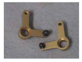
Assemble the control system; starting with the collective arms (popsickle sticks), aileron bellcranks, and "X" arm. Install the short balls in all of the pieces, using loctite, making a right and left aileron bellcrank as shown. Install the 5X8X2.5 flanged bearings into the pieces, putting 1 ea into the popsickle sticks, and 2 ea into each bellcrank.
