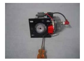
You'll want to remove that sharp edge, either by buffing or carefully grinding the edge. Install the pull start adapter using 3 ea 5X12 FHCS. Loctite is NOT necessary here, as the countersunk G10 will hold them quite nicely.
