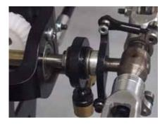
Make sure the ball on the servo wheel is straight down, then adjust the length of the pushrod to center the tail pitch slider on the output shaft as shown.
