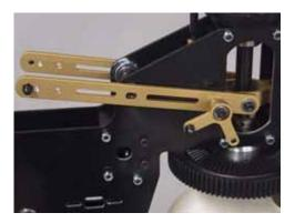
Install the left side popsickle stick, matching the broach in the popsickle stick to the flats on the collective axle, using a 3X4 SHCS and 3M washer at the front into the shaft for the elevator yoke, and a 3X8 SHCS and 3M washer into the collective axle. The right side popsickle stick is installed the same way, except,
