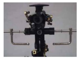
Flybar installation is next. Insert the flybar through the seesaw tube bearings; install a 4mm special washer on each side, then the flybar arms.
