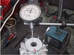
Dial indicate the fan, looking for runout indication as shown.
