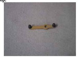
Note the orientation of the balls on the "X" arm. Install 2 short balls on the elevator bellcrank, with loctite.
