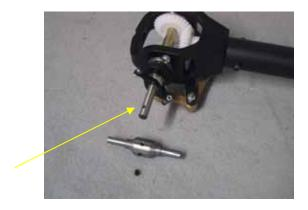
Slide the pitch slider onto the shaft engaging the ball into the delrin cup at the same time. Locate the Heavy Duty tail hub and 1 ea 3X4 setscrew. Note the divot on the output shaft.
