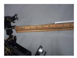
Install the flybar paddles onto the flybar, counting at least 20 turns on, measuring both sides from the flybar arm to the paddle, to ensure they are the same dimension. Use the front hole in the paddle. Also level the paddles with each other, as viewed from the end.
