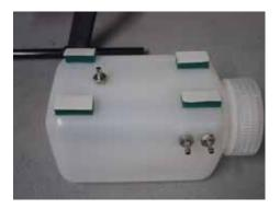
Secure all fittings with a nut on the outside. If necessary, you can seal the holes under the fittings with Zap-a-dap-a-goo or similar glue. Install the lid tightly. Install some sort of padding on top of the tank; we use Zeal anti vibration gel, which is a double sided adhesive.
