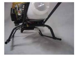
Install the boom assembly into the boom clamps at the rear of the frames, pushing it all the way in to engage the dogbone into the delrin cup. Once engaged, pull back 1 mm to relieve any pressure on the drive train. Attach the boom supports to the bottom of the frames using 2 ea 3X10 SHCS and 3M locknuts.
