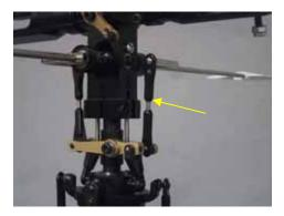
The pushrods from the aileron bellcranks the swashplate are 60 mm long, center to center, using the 40 mm long pushrods. The pushrods from washout arms to flybar arms are 48 mm long, center to center, using the 30mm long pushrods.
