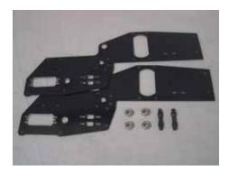
Install the clutch system onto the delrin bushings on the fan hub. Gather up the upper frames, 4 ea flanged bearings, and collective axles.
