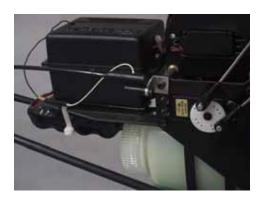
We also recommend a base loaded antenna, such as the Revolution brand shown here, available from Horizon Hobbies. We also have the angle brackets shown to attach them to the framework. We recommend using a Strongbox for your receiver from Sonic-Tronics, also available through us at Bergen R/C. Either way, attach your receiver and battery packs securely to the battery tray using padding and tye-wraps or Velcro.
