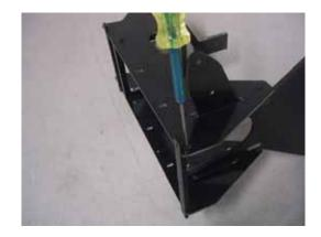
Install the rear bulkhead using 4 ea 3X16 SHCS and 3M locknuts, then install the landing gear skid bars, front and rear, using 4 ea 3X8 FHCS.
