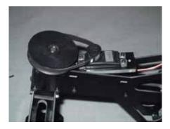
Install the small pulley/servo wheel onto the servo, then place one of the servo assemblies in between the extension arms, angling it in while installing the pulley belt.
