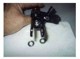
Locate your thrust bearings for the blade grips. Notice that one of the races has a larger inner diameter than the other. Grease the ball cage, then install the larger ID race inside the blade grip, on the head axle, with the groove facing out.
