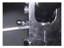
Slide the head assembly onto the main shaft, lining up the "jesus" bolt hole with the hole in the mainshaft. Slide the pins from the washout unit up into the slots in the head.
