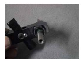
Install 2 ea 3X5 panhead screws to secure the bearings in the headblock, being careful not to get any loctite in the bearings. Insert the head axle into the head, and push some grease into the gap around the head axle, on both sides of the head. This acts as a reservoir of lubrication for the dampening o'rings.
