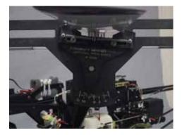
For pitch setup we offer a flybar lock with flag or use your favorite method of centering the flybar. Place a pitch gauge on one of the blades. Pitch setup is a personal preference thing, but here's our suggested pitch range.
