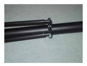
Thread the ends into the boom supports using JB Weld to secure. Let dry overnight, making sure the ends are parallel with each other while they dry. After drying, attach to the horizontal fin clamp, using a 3X30 SHCS, 2 ea 3M washers, and a 3M locknut. Don't tighten yet.
