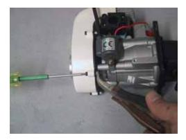
When you get all 4 SHCS installed, warm the entire shroud to relieve any stress that could cause cracks in the future. Install 4 ea 3M locknuts on the SHCS. DO NOT over torque these nuts; you will crack the ears on the first run of the engine. Snug is good enough.
