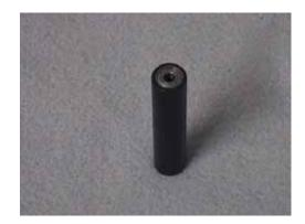
Assemble the rotor head next, starting with the seesaw. Press 2 ea 4X10X4 bearings into the end of the seesaw tube until flush. Be careful not to confuse these bearings with the 3X10X4 bearings used later. The bearings you want have the larger inner diameter.
