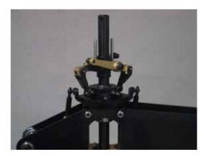
Slide the completed assembly onto the mainshaft, and snap the porkchops onto two of the inner balls of the swashplate.
