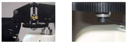
Continue pushing the main shaft down, through the bottom bearing, insert the main gear below the bottom bearing block and slide the main shaft through the auto hub. Place the bottom collar on the main shaft and install the 4-40 bolt through the collar and mainshaft, with loctite. This is one of the 2 standard, not metric, bolts on this helicopter.
