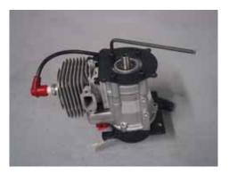
Install the pull start using 4 ea 4X12 SHCS. Again, loctite isn't needed, however if you feel the need, you can use a drop of CA glue in place of loctite. Note the orientation of the pull start handle, on the same side as the carburetor insulator block. On the opposite end of the engine, install the fan shroud mount plate, using 4 ea 5X12 SHCS and loctite this time. Also note the orientation of the plate; this will be important when you mount the fan shroud.
