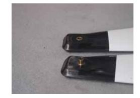
Install the NHP 800 MM Blades, first inserting the brass bushing into the root.
