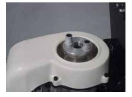
Locate the delrin bushings, steel inserts and 4X16 SHCS. Note the chamfer on the steel insert. Install with the chamfer toward the head of the bolt. Install the delrin bushings onto the fan hub using loctite, and tighten securely.
