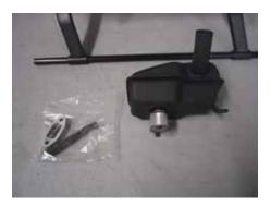
Install the muffler next. Note that there are 2 spacers and 2 sets of bolts. Use the thicker spacer and the longer 5X65 MM set of bolts. Install a gasket on either side of the spacer, put the bolts through the muffler and spacer assembly,
