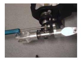
Locate the 4M shoulder bolts and eyelets. Slip the eyelet onto the shoulder bolt and install on the blade grip with loctite, being careful not to get loctite into the eyelet. It has to rotate on the shoulder bolt to operate properly. If you run into tail problems, drift, hot servo, tail wont hold, look here as a possible culprit. You should also lubricate this joint daily with a light lubricant such as 3 in 1 oil.
