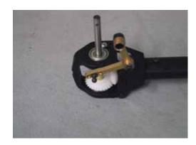
Thread a 3M locknut onto the bolt and set the tension on the bearings by tightening the bolt, then tightening the nut to secure. Check that the bellcrank spins freely with minimal slop. If further adjustment is needed, loosen the nut, adjust the bolt, then retighten the nut.
