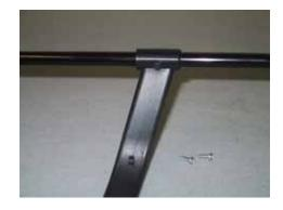
Install the lower frame assembly onto the landing gear, using 4 ea 3X16 SHCS and 3M locknuts. Center and rotate the skid tubes to your liking, then drill a #50 pilot hole in the boss, into the aluminum skid tube, on the underside of the gear and install the 2 ea 3X8 self tapping screws. I typically install these into the rear cross bar, leaving the front crossbar able to flex.
