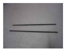
Locate 2 ea arrow shafts, they are aluminum, and you will see a silver dot on each end. Cut 1" off of each end of both arrow shafts. This is to remove the part of the arrow shaft that is not machined to the proper size. Now cut 1 arrow shaft 16 <sup>1</sup>/<sub>4</sub> " long, the other 17" long.
