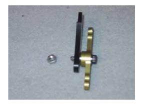
Insert 2 ea 3X7X3 flanged bearings into each bell hiller mixer, then insert a 3X12 SHCS with 6M shoulder and place a 3M brass washer on the threads. Thread this assembly on to the pitch arm in the center hole, noting the orientation of the flat milled on the pitch arm. Set the tension on the bearing by tightening the bolt carefully, then installing a 3M nut with loctite as a jamnut. The arm should spin freely with no slop.
