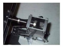
With the spacer installed, slide the long upper shaft into the thrust bearing block and install the thrust bearing that consist of 2 races with a ball cage in between. Install the third split collar onto the shaft, noting the orientation, ring down.
