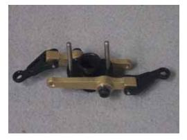
Thread the bolt into the washout hub, then install a 3X4 setscrew in the same hole from the opposite side. Set the tension on the bearings by tightening the bolt carefully until the arm spins freely, but there is no side to side slop. Tighten the setscrew, using it as a jamnut to secure the bolt. Check the play on the arm. If it changed, loosen the setscrew, and readjust, tightening the setscrew when done. Repeat for the opposite arm. Install a short ball onto the inside of each arm.
