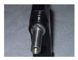
Install 2 ea o'rings on both sides of the head on the axle, and push them into the head. Now you install the dampening shims. Here you have a choice. You must install the thickest of the three shims (.040), but can install one or both of the other shims (.008, .015) to suit your flying. Then push on the circlip until it pops into the groove in the shaft. Make sure it's seated all the way around.
