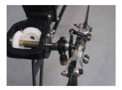
With full rudder stick, adjust the travel on the pot on the gyro to give full travel without bottoming out on the gearbox or tail hub. The travel should end up being between 100 and 120 on the gyro. If not, change the position of the ball on the servo in or out as needed to get between 100 and 120.
