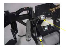
Install the Vibration Isolators onto the "Flying Squirrel" using 8 ea 4X12 SHCS threaded into the G10, then install the completed camera mount assembly onto the vibration isolators using 4 ea 8-32 SHCS.
