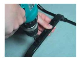
Start with the landing gear. Assemble the skids and cross bars as shown, leaving them loose for now. Locate the landing gear skid bars in bag #1, use them to locate and drill 2 holes in each cross bar. Center the skid bar fore and aft, as well as side to side, and use a #30 or 1/8<sup>th</sup> drill bit to drill through the cross bar. Set the landing gear aside for now.
