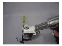
Set the fan shroud over the fan and head of the engine. Carefully, using a hair dryer, warm the shroud to fit it to the mount, installing the 3X16 SHCS as you go.
