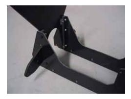
Using 6 ea 3X16 SHCS and 3M locknuts, mount the bars on the butterfly, then slide the one leg into the lower frame, again using 3X16 SHCS and 3M locknuts through the "front frame plate bar" to secure in place. Repeat for other lower frame half. Note that the lower frames are "handed", left and right. You can tell the difference by the countersunk holes on the lower edge of the frame. The countersink faces
