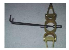
Note the two shafts are different; one has flats on only one side. Install both shafts into the elevator yoke with the flats fitting into the broached holes. Use loctite on the 2 ea 3X4 SHCS and 3M washers.
