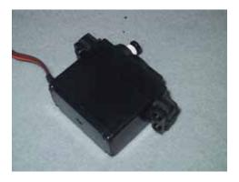
Secure the servos with screws provided with JR servos, or if using Futaba servos, use 2.5X10 SHCS and 2.5M washers. These screws and washers are available from Bergen R/C. The collective servo uses the plastic servo mount tabs installed in the rubber grommets, as shown.
