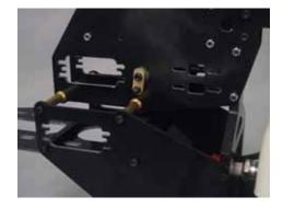
Install the triple bellcrank on the left side, on the collective axle, matching the broach with the flats on the axle. The single bellcrank is installed on the right side, on the collective axle. Use 2 ea 3X8 SHCS with 3M washers and loctite. Note that the legs with the short balls on both bellcranks should point in the same direction, as shown, both are pointing down.
