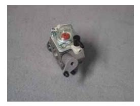
On the carburetor you will find an idle adjustment screw, remove it and throw it away. Install the throttle arm on the carb, in the direction shown. With the carburetor butterfly halfway open, you want the throttle arm pointing straight away from the carb. The idea here is to center the throw of the arm for setup purposes.
