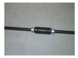
Install the long arrow shaft onto the input shaft of the gearbox, using a collar with only 1 ea 3X3 setscrew to secure. Install the bearing carrier and coupler onto the long shaft and install the shorter shaft on the opposite end, again securing with a collar and only 1 ea 3X3 setscrew on each shaft.
