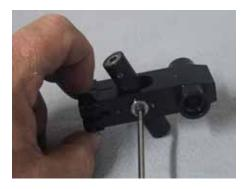
Now use the 3X10X4 bearings, a 3X8 SHCS and 3M brass washer, Insert the seesaw tube into the oval hole in the head, and thread the bolt into the seesaw tube. Use the bolt to draw the bearing into the head. Note the orientation of the slots on the seesaw tube, and use loctite on these bolts.
