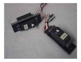
Snap the plastic servo mount tabs into the slots in the servo mounts, noting the orientation. Install the servos into the mounts using 2.5X10 SHCS and 2.5m washers, which thread into the plastic servo mount tabs.
