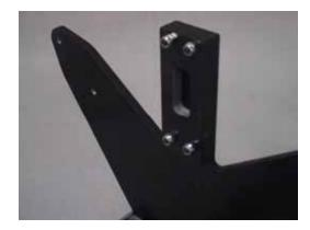
Install the battery tray into the frames using 4 ea 3X8 SHCS and loctite. Note the tray spacers are on top. Install the "Front Frame Block and Arm Mount" on the rear of the butterfly, using 4 ea 3X16 SHCS and 3M locknuts.
