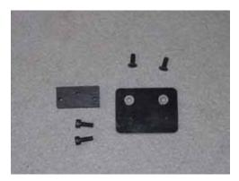
Install 3 sets of the boom clamps into the rear of the upper frames, using 6 ea 3X35 SHCS and 6 ea 3M locknuts, but do not tighten them yet. Locate the gyro mount plate and three hole block.
