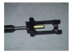
Secure the cross pin with a 3X4 setscrew threaded into the rear of the shaft, using loctite. Make doubly sure the setscrew secures the crosspin. Insert the shaft into the rear of the transmission cradle through the bearing, and slide the brass tube onto the shaft.
