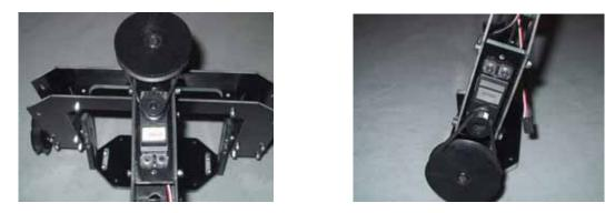
Push the servo mount in until the thru holes line up and install 2 ea 3x35 SHCS, 4 ea 3M washers, and 2 ea 3m locknuts. Set the tension on the belt fairly tight and tighten the nuts. Repeat for the tilt servo on the side of the turret arm.
