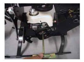
Fit the air filter base to the carb, with a gasket between them, inserting the attach bolts through the base and carb. Install a gasket on the open face of the carb also. Bolt this assembly to the insulator block on the engine, being careful not to overtighten, as this will distort the insulator block causing air leaks and lean runs on the engine. The choke lever should move with some resistance.
