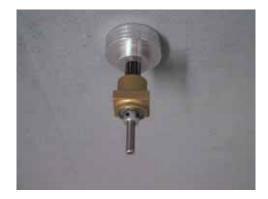
Assemble the clutch components, clutch, clutch bell, triple bearing block, and retaining collar w/3X3 setscrews. Use loctite on the setscrews in the retaining collar.
