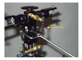
The pushrods from the seesaw to bell-hiller mixer require trimming of the ball link, cut 1/4" off of the end and thread onto the 3X12 setscrew. The length will be 30 mm from center to center.
