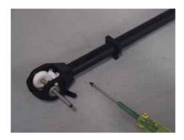
Lubricate the O'rings on the bearing carrier, and slide the complete assembly into the tail boom. Secure the gearbox into the boom with 2 ea 3X4 SHCS and loctite. Be careful not to overtighten these screws as you can pull the threads out of the gearbox, use the loctite and they will stay secure.
