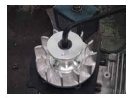
Installing and dial indicating the fan will be more accurate with the spark plug removed. Seat the fan on the tapered end of the crank, and install the 6X25 SHCS and <sup>1</sup>/<sub>4</sub>" split washer, using loctite. Do not torque the bolt down yet, just snug it.
