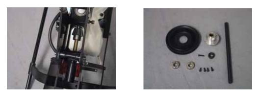
Install the tail transmission into the upper frames, engaging the ears into the lower bearing block. In these "ears", note the slotted hole for adjustment up and down to set the mesh. You'll need to remove the 3X35 SHCS previously installed, the reinstall it after getting the transmission in place. Don't tighten it just yet. Loosely install 4 ea 3X8 SHCS into the rear 4 holes of the cradle through the frames. Locate the main gear components next.
