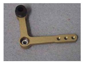
Assemble the tail pitch bellcrank by installing a 3X7X3 flanged bearing in one side, the aluminum spacer,
