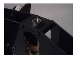
Install the lower main shaft bearing block, using 2 ea 3X35 SHCS, note the orientation of the bearing, facing up. The elevator yoke is removed for clarity. Install the upper main shaft bearing block, using 4 ea 3X8 SHCS also note the orientation of the bearing, facing down this time, hump side up. Loosely install 2 ea 3M locknuts on the lower bolts.
