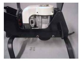
Install the engine into the lower frames, spark plug facing to the rear (remove the plug for ease of installation). Note the vertical slots in the lower frames and the horizontal slots in the pull start adapter. In these slots, install 4 ea 3X18 SHCS with the thick special washers provided, one washer on the outside, one on the inside.
