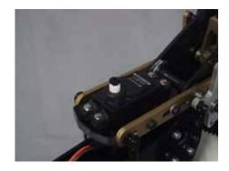
The collective servo is installed between the frames, with the spline to the rear. The aileron servo is installed on the mount between the collective arms, spline to the rear.
