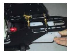
Install the fuel tank, starting with locating where the fuel fittings will be installed in the tank. Slide the tank under the battery tray and mark where you want the fittings.
