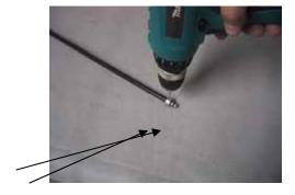
Install the "dogbone" assembly in the front end of the short arrow shaft, again with a collar and only 1 ea 3X3 setscrew to secure. Using a #50 drill bit, pick one hole in each collar and carefully drill through the arrow shaft into the underlying shaft or dogbone, creating a divot in the shaft. With loctite, install a 3X3 setscrew in each drilled location. Remove, loctite, and reinstall the rest of the setscrews in each collar.
