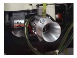
As an option, we offer a velocity stack for your carb, doing away with the somewhat restricting air filter. If you are flying in a dusty area, we do not recommend this. You also lose the choke function built into the air filter, but you can get a carb with the choke built in, as shown.
