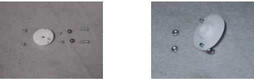
When you have each wheel marked, put a ball on a 2X10 Phillips screw, thread a 2M nut up to the ball, then screw the assembly into the wheel at the marked hole.
