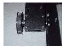
Push the assembly all the way up, push the split collar down on top of the thrust bearing and tighten the split collar bolt, NO loctite. The camera mount should spin freely. Install a large pulley onto the shaft, installing a 3X20 thru bolt and 3M locknut. You may need to tap up on the whole assembly to get the holes to line up, then carefully tap it back down. Now tighten the bolts securing the bearing blocks to the extension arms.
