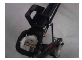
Adjust the length of one special ballink until both blades touch the bolt when rotated. Now check your travel limits again to see if adjustments are needed.
