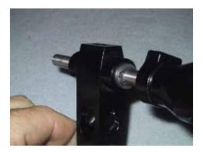
You may need to use the blade grips to push the circlips into place, just make sure they are seated all the way around. Now slide the blade grips onto the head axle, all the way to the circlip.
