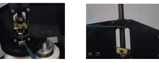
Pull up on the mainshaft, push down and tighten the lower split collar. This is where the hardened allen drivers are a must. You'll notice the heads of the bolt are turned down to fit the collar, making them very easy to strip the heads. Slide the upper collar and thrust bearing up to the upper bearing and secure the bolt. DO NOT use loctite on these bolts.
