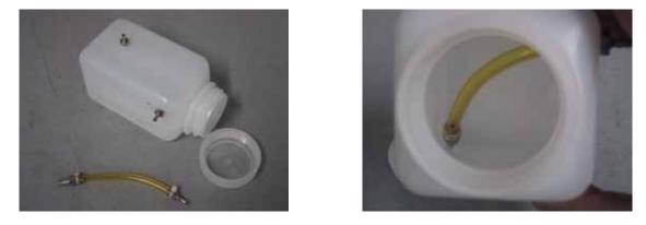
Drill a #16 hole in the tank at the spots marked. Install a single end fitting on the top of the tank for the vent line, and one on the side for the return line. Make a clunk line using the double end fitting and clunk securing the ends with a tye-wrap, making sure the line is long enough to reach the bottom of the tank, but not too long to get stuck in the corner.
