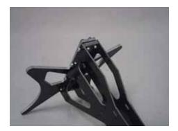
Place an extension arm on one side, and install 4 ea 3X35 SHCS through the Front Frame Blocks, then place the opposite extension arm on the bolts and thread 4 ea 3M locknuts on the bolts. Now tighten all the bolts, pulling the extension arms up to the "flying squirrel" tightly.
