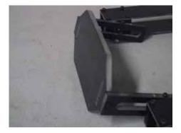
Install the height adjustment arms onto the shafts, putting a 3X30 SHCS through the arm and the hole in the shaft, securing with a 3M locknut. The three different holes allow for height adjustment when using different sized cameras. Install the base plate in between the arms securing with 4 ea 3X20 FHCS and 3M locknuts. Slide the split collars toward their respective bearings and tighten. DO NOT use loctite on these split collar bolts.
