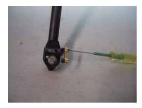
Then the opposite bearing. Insert the 3X16 with 6M shoulder SHCS through the bearings and spacer, with the delrin cup on top, and add a 3M brass washer on to the bolt as a spacer. Thread this into the pitch arm on the gearbox, but do not tighten yet.
