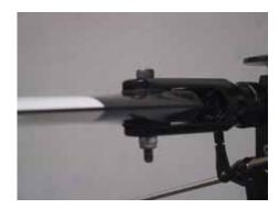
Put a plastic spacer on each side of the blade root and slide the assembly into the blade grip. Note direction of rotation, in this case, clockwise as viewed from above the rotors. Install a 4X25 SHCS w/shoulder through the assembly and secure with a 4M locknut. Tighten the blade bolts enough that the blades will not fold when the heli is turned on its side and shaken.
