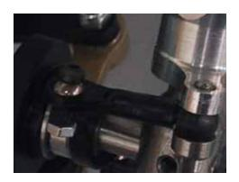
Thread the Special Ball Links onto the eyelets and snap onto the balls on the pitch slider. Note direction of rotation as shown.
