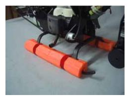
You can install Pool Noodles on the landing gear as a visual aid; you may need to divert the exhaust as shown to prevent melting the foam.
