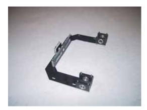
Through one turret arm, install 12 ea 3X35 SHCS and place flat on the table. Install 1 ea "G10 block with 10m hole", one ea "Extension Arm and Turret Brace", and 4 ea standard bearing blocks onto the 3X35 SHCS. Note the orientation of the bearing blocks.
