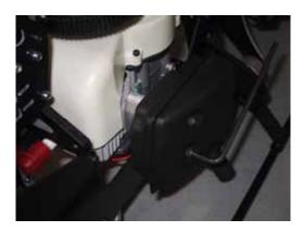
And bolt to the engine. Point the exhaust tube down. After the first run of the engine, go back and tighten these bolts while the muffler is still hot.
