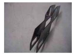
Press the flanged bearings into the upper frames, making certain to seat the flange down. Be sure to make a right and a left, with the flange on the inside of the frames. Put a drop of CA glue around the outer edge of the bearings to secure them in place, being careful not to get any glue in the bearing itself. Insert the axles into one side frame and slide the opposite side frame onto the axles.
