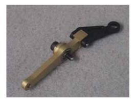
Insert the 3X7X3 flanged bearings into the arms, 2 ea into each arm. Insert the 3X16 SHCS with 6M shoulder through the bearings and put 1 ea 3M brass washer on the bolt. Note the orientation.
