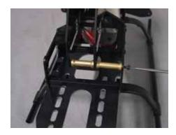
Gather the 26 mm threaded frame spacers and 29 mm non-threaded frames spacers with 4 ea 3X40 SHCS. Secure the rear of the frame sets together by inserting the bolt through the frames and spacer, into the threaded spacer in the middle.
