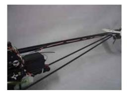
Install Gyro on the mounting plate, preferably with the green Zeal anti vibration gel, and connect to servo and receiver. Use a long servo extension wire to connect the servo to the Gyro, securing the connections with tape or heatshrink.
