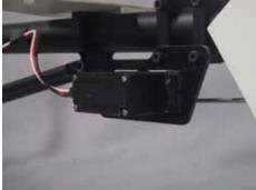
Install tail rotor servo into rear mount plate with spline forward.
