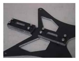
Begin assembling the camera mount by installing the Front Frame Block and Arm Mounts to the "flying squirrel", noting the orientation, with 8 ea 3X16 SHCS and 3M locknuts. Don't tighten these just yet.
