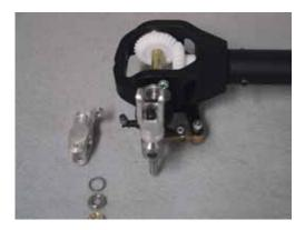
Install 1 blade grip, then the 10m spacer. The thrust bearings include 2 races and 1 ballcage. One of the races has a larger inner diameter than the other. Install this race next, then the ballcage after greasing. The race with the smaller ID is next, then is secured with a 3X6 SHCS and 3M washer with loctite. There will be a small amount of in and out play, this is normal and designed in to the system. Repeat for other blade grip.
