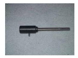
Assemble the tail drive transmission next. Insert the shaft into the delrin coupler until the holes line up and install the cross pin securing the two pieces together.
