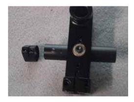
When both bearings are installed, center the seesaw tube by tapping on the head of the bolts. The seesaw tube should pivot freely. Install the seesaw tube endcaps, pushing them on until flush with the end, and securing with a 3X4 setscrew and loctite, in the inner hole. The setscrew should engage the slot on the tube. Also install the short balls in the outermost hole at this time.
