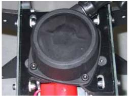
Turn the framework over to access the underside, and install the washers and 3M locknuts. Do not tighten at this time, as you will need to set the gear mesh later on. Note that you can move the engine up and down, as well as forward and aft.
