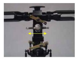
Center the flybar, measuring both sides from the flybar arm to the end, with the flybar arm pushed all the way to the seesaw tube. Secure the flybar arms with a 3X4 setscrew and loctite, making sure the flybar arms are parallel with each other.
