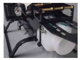
Install the tank under the rear tray and secure with the 2 long tye-wraps provided, running the tye-wraps through slots in the tray.
