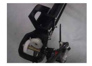
To static track the tail blades, try this. Fold both blades up against the blade grips. Push one blade in until it touches the bolt for the vertical fin mount. Without changing the pitch, carefully rotate the tail system until the opposite blade comes close to the same bolt.
