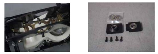
Insert the elevator yoke into the upper frames, with the longer of shaft on the right side of the helicopter. Find the 2 main shaft bearing blocks. Note the cutout portion on the lower bearing block.
