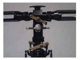
Install 2 ea short balls on the mixers. Note that one end of the arm is longer than the other, and orientation of the balls. In this instance the longer end is to the right. Install the assembly onto each blade grip using 2 ea 3X6 SHCS and loctite. The milled flat on the pitch arm should square up the pitch arm to the blade grip.
