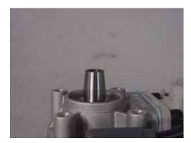
Gather all of the engine components. Note the tapered end of the crankshaft. Also notice the sharp edge at the end of the taper.
