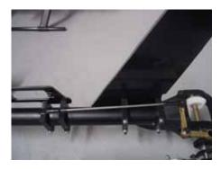
The tail servo mount is installed between the vertical and horizontal fins using 2 sets of boom clamps, and 4 ea 3X30 SHCS and 4 ea 3M locknuts. It's position will be adjusted after installing the servo. The push rod can be installed also, but will need to be adjusted later as well. Use the 140mm pushrod.
