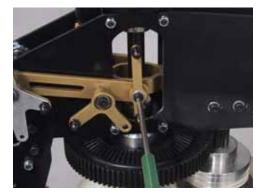
The "X" arm bolt threads into the collective axle, setting the tension on the bearings by holding the jamnut, then tightening to the popsickle stick. Install the elevator bellcrank onto the long shaft of the elevator yoke, matching the broach to the flats on the shaft. Use a 3X4 SHCS and 3M washer with loctite. The long leg of the bellcrank points up.
