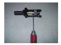
Install the tail pinion onto the shaft and slide the shaft all the way in, through the forward bearing. Looking through the setscrew hole, locate the divot in the shaft. If it doesn't line up, look through the second hole in the pinion. Install a 3X4 setscrew in this hole, using loctite. A second setscrew is not necessary and may interfere with the bolts in the main gear.
