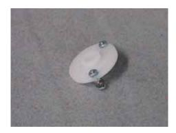
Thread another 2M nut on the backside of the wheel securing with loctite. Repeat for all the other wheels, with the throttle and tail servo wheel only using 1 ball on each. Turn on the radio system again, making sure each servo is centered and reinstall the servo wheels onto the servos. Don't forget to put the servo wheel screws in!
