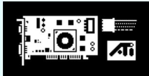
flashing red power connector will appear on your display and the computer will not start if the RADEON 9800 PRO Mac Edition is not correctly connected to the power supply.
