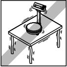
Place the scale on a stable surface which is free of vibrations and as horizontal as possible.
