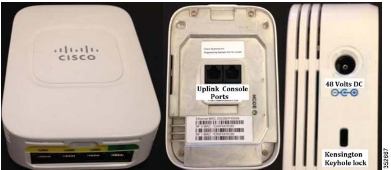
Figure 3 AP-702 Ethernet Switched Ports
