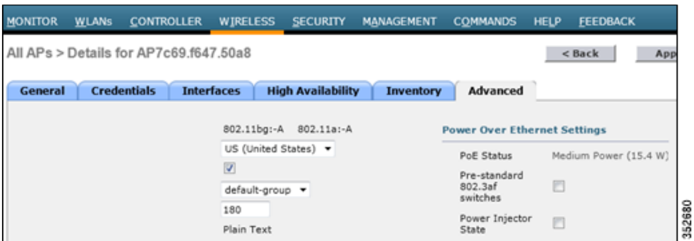
Figure 15 PoE out on Port 4 will not happen if PoE Status is only Medium Power (15.4 W)
