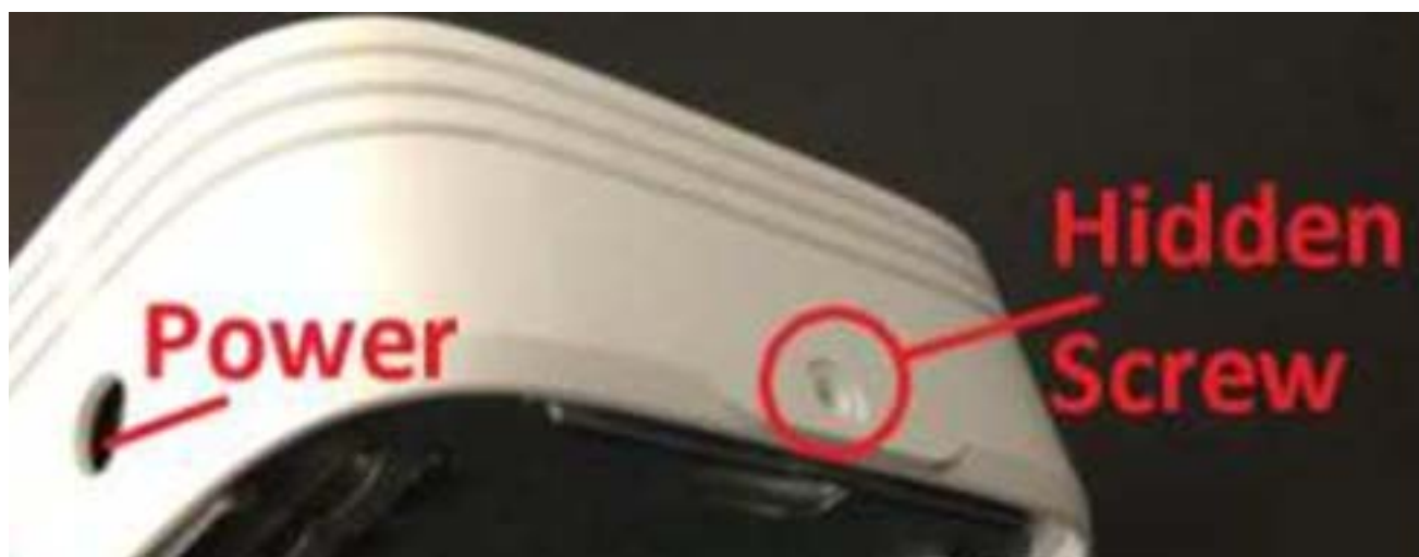
Figure 4 The AP may be secured into the bracket with a hidden tamper resistant screw
