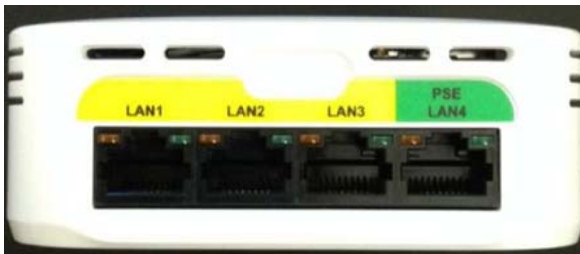
Figure 14 Ethernet Switched Ports AP-702W
