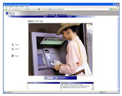
The **Decoder connection** page will be displayed as the home page for a receiver. It shows a snapshot from the video source for the sender currently connected, and the unit searches the network automatically for available senders.
