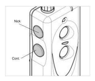
The transmitter for *dogtrd 1800NC* has two buttons. The top is the Nick button and the bottom is the Constant button.
