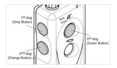
The transmitter for the *dogtrd* 1803NC has three buttons; The Gray (1st dog) button corresponds to the receiver with the black collar strap. The Orange (2nd dog) button corresponds to the receiver with the orange collar strap. The Green (3rd dog) button corresponds to the receiver with the green collar strap.
