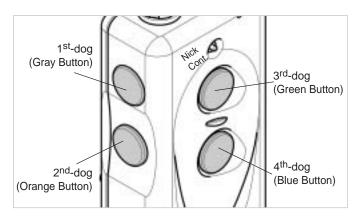
The transmitter for the *dogtra* 1804NC has four buttons; The Gray (1st dog) button corresponds to the receiver with the black collar strap. The Orange (2nd dog) button corresponds to the receiver with the orange collar strap. The Green (3rd dog) button corresponds to the receiver with the green collar strap. The Blue (4th dog) button corresponds to the receiver with the blue collar strap.
