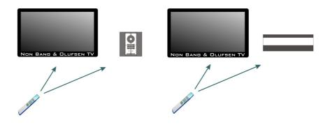
If there is a Bang & Olufsen audiomaster in the room, it can be used for handling the sound. Speakers connected to an audiomaster are of a much better quality than the speakers in a TV. In a B&O linkroom setup with Beolink Active or Beolink Passive, you can also use these speakers to improve sound from most TV's.
