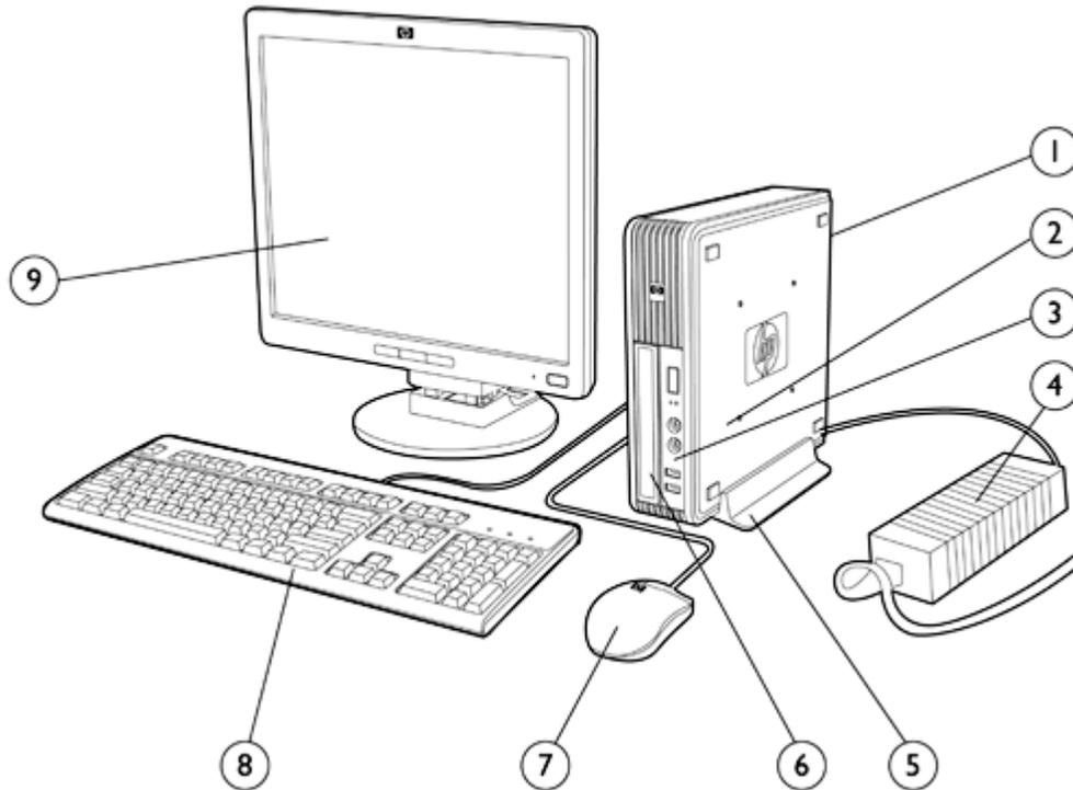
1. Rear I/O: (6) USB 2.0, (1) DisplayPort, (2) PS/2, (1) RJ-45, (1) VGA port, (1) audio in, (1) audio out
