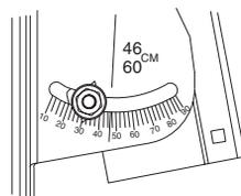
If you have the bracket where the edge of the mast shows through the curved slot, align the edge with the desired elevation mark.
