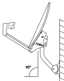
5. Place the dish on the support arm. Align the flathead bolts with the dish support bolt holes on the dish supports.
