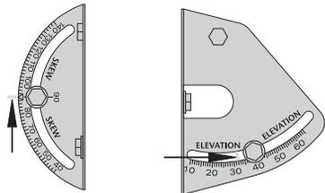
Line up the red notch with the correct angle on the skew scale.
