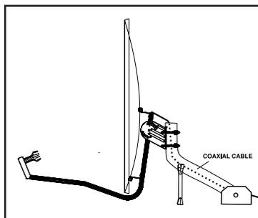
4. **Attach the LNBF to the LNBF cable(s). Slide the weather boot up securely to cover the cable/LNBF connection at the base of the LNBF.**
