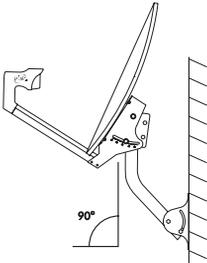
The figure above shows how you should attach the mast to the foot for mounting on vertical surfaces.
