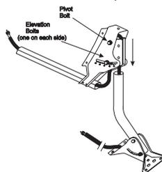
10. Turn the antenna mount on the mast or pole to align the LNBF support arm in the direction of the satellite. Use the direction you found earlier in the Satellite Location Reference Chart.
