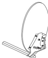
8. Tilt the support bracket to the approximate elevation of the satellite. Use the elevation you found earlier on the Satellite Location Reference Chart.
