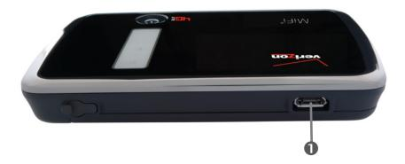
**1** Micro USB Connector: The wall charger connects here.
