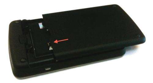
**4** Connect the Micro USB end of the wall charger to the Micro USB port on the device.
