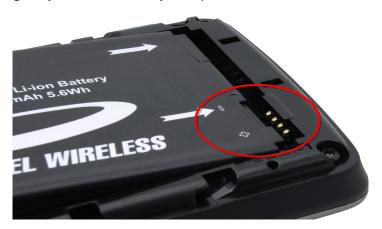
**3** Replace the cover by setting it on the device where the notches align, and then gently slide the cover back toward the release button until it clicks into place.
