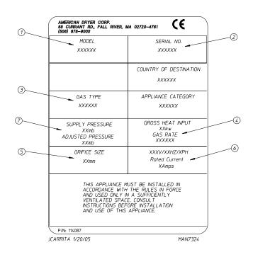
When contacting ADC, the information on the data label is required to ensure proper service/parts assistance. The data label is located at the upper left rear of the dryer behind the back guard.
