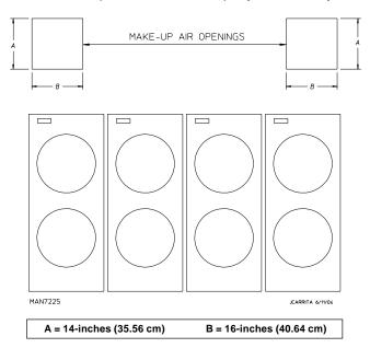
EXAMPLE: For a bank of 4 SL3131 dryers, 2 unrestricted openings measuring 14-inches by 16-inches (35.56 cm by 40.64 cm) are acceptable.
