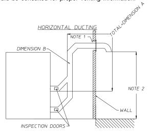
A = SL2020/SL2929 - 20 feet (6.10 meters) SL3131 - 12 feet (3.66 meters)
