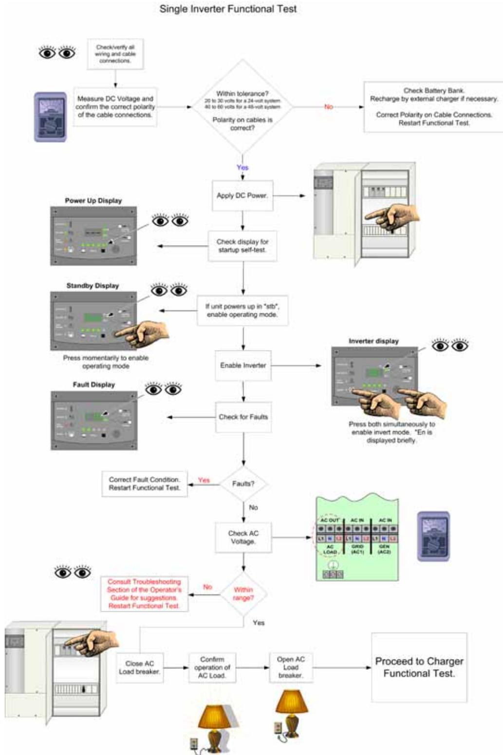
Figure 2-26 Functional Test for Single Inverter Systems
