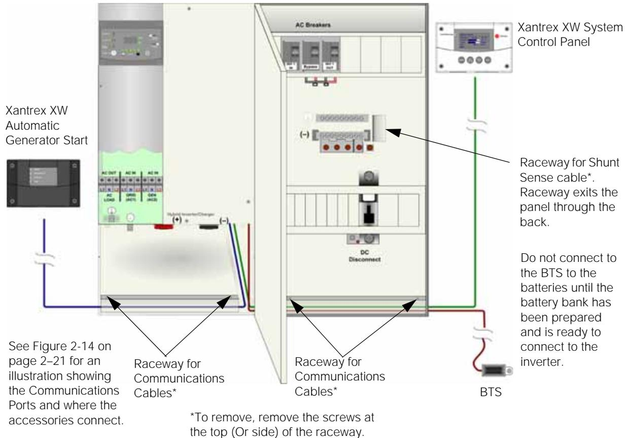
Figure 2-8 Routing Communications Cables
