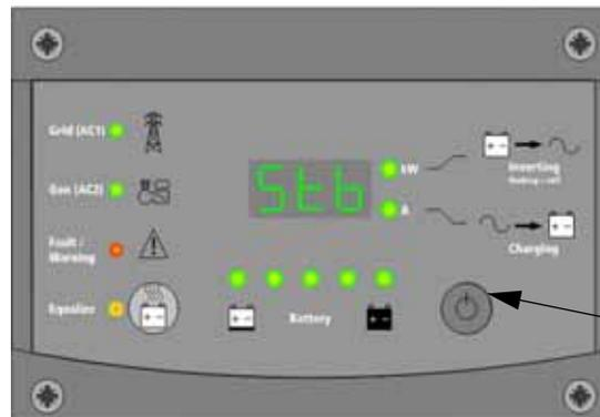
Note: If the inverter was previously powered up then it will power-up in the last operating state (Operating or standby)
