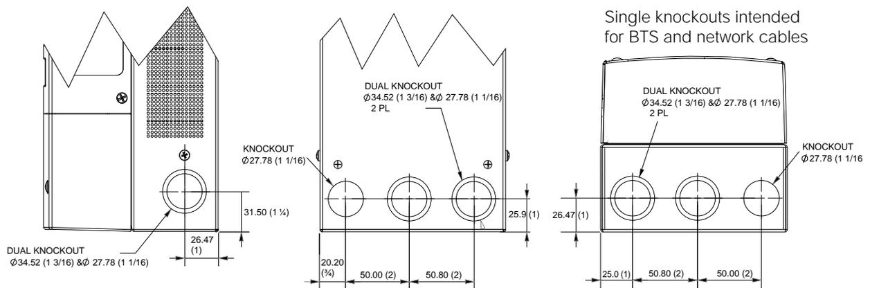
Figure 4-4 Knockout Dimensions
