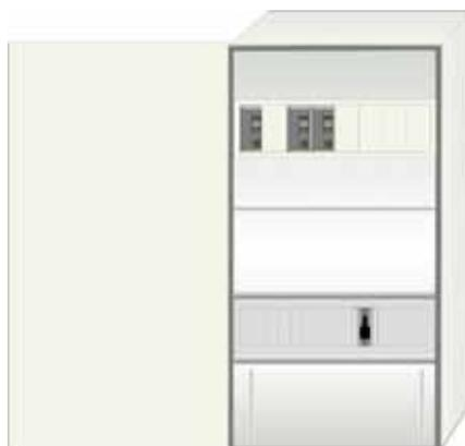
The panel door can be mounted on the right or left side of the Xantrex XW Power Distribution Panel.
