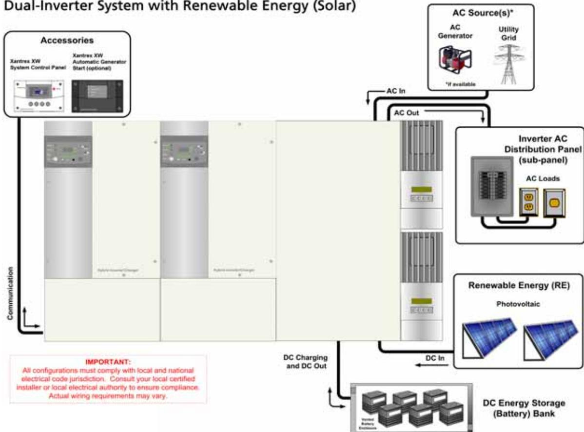
Figure 1-1 Xantrex XW Power System Installation Diagram Example
