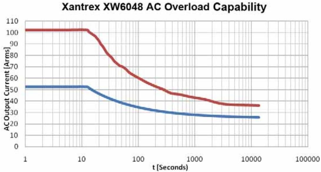
Figure A-1 Xantrex XW Series AC Overload Capability
