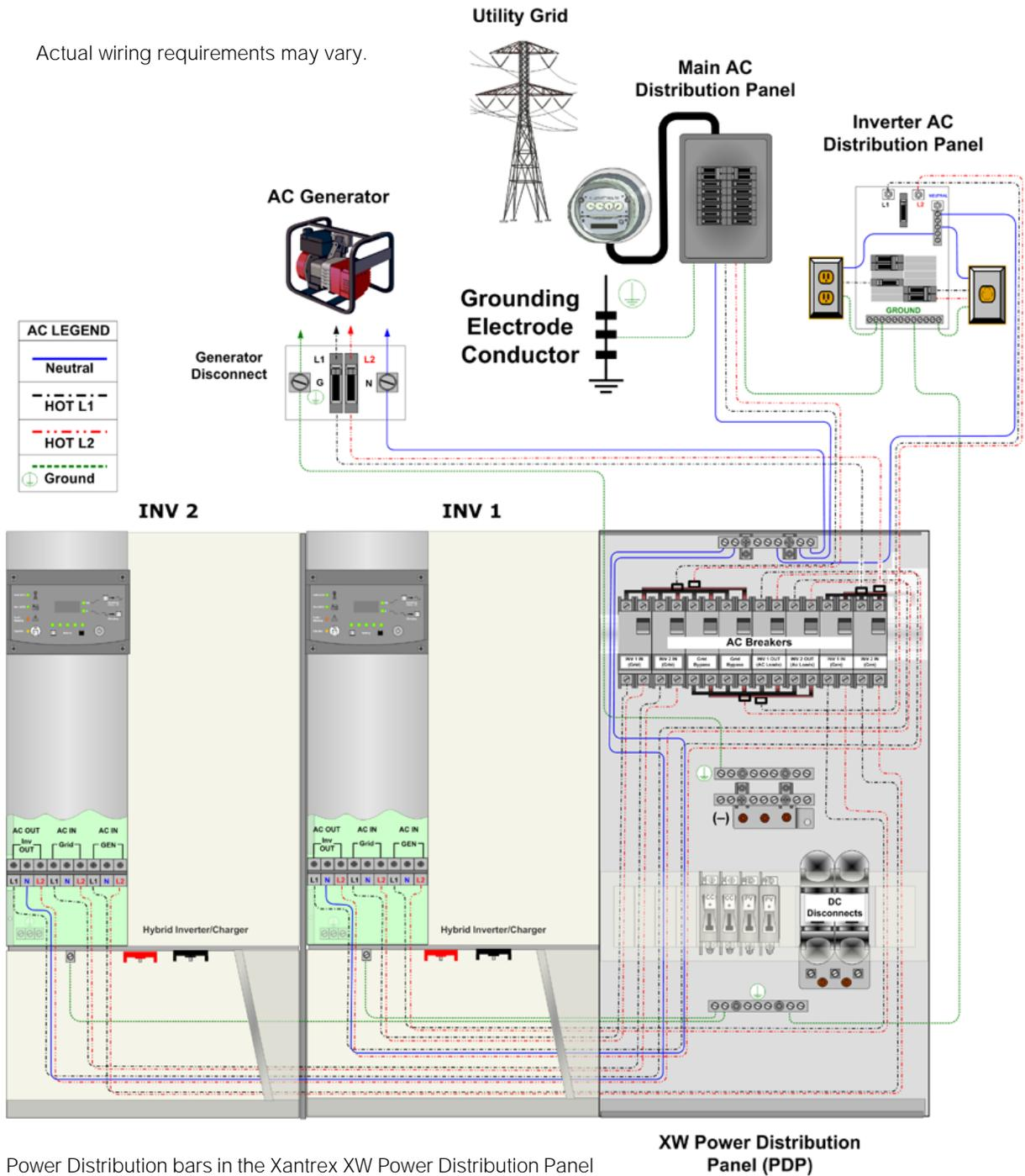
Power Distribution bars in the Xantrex XW Power Distribution Panel accept up to a #2/0 AWG cable (maximum). See Figure 2-9 on page 2-14 for torque requirements.
