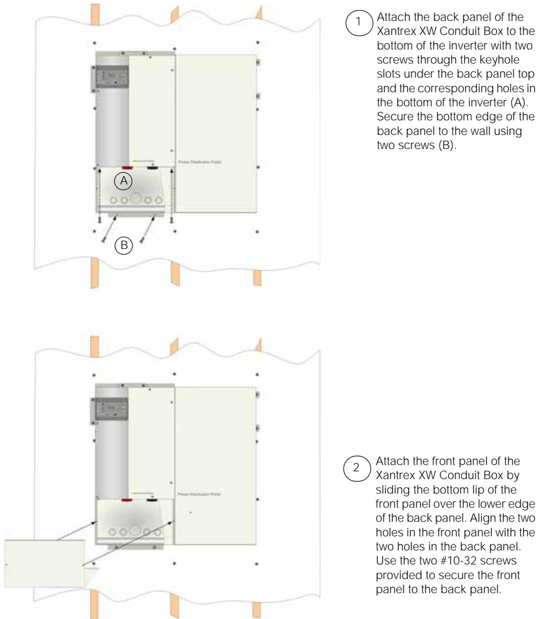
Figure 2-7 Installing the Xantrex XW Conduit Box
