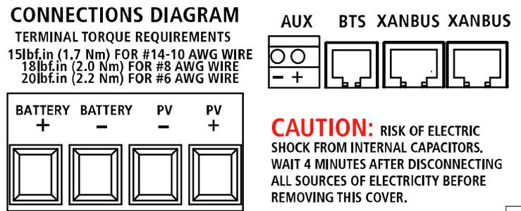
Figure 4-8 DC Connection Terminals
