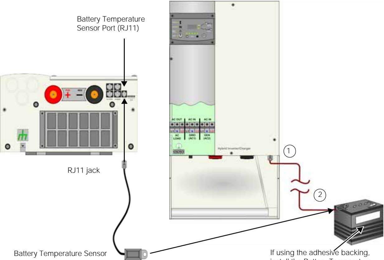
Note: If other Xantrex Xanbus connected components supply a BTS or are BTS enabled, it is not necessary to install all of them at once. Only one BTS needs to be installed.
