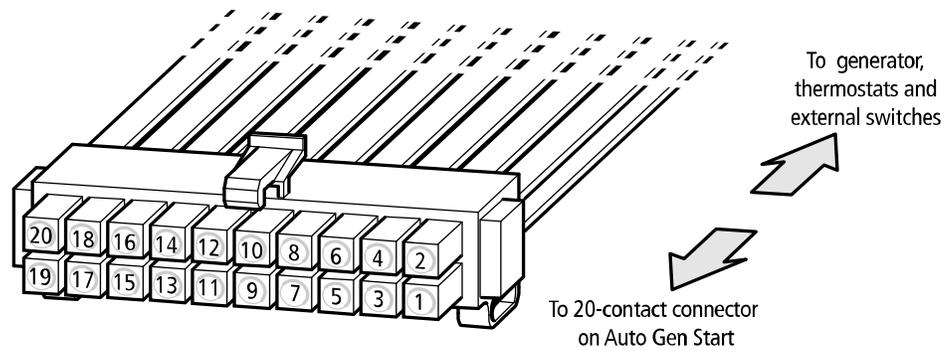
**Figure 5-9** Xantrex XW Automatic Generator Start Wiring Harness
