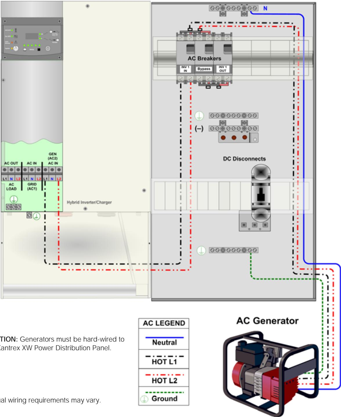
**CAUTION:** Generators must be hard-wired to the Xantrex XW Power Distribution Panel.
