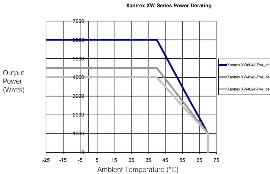
Figure A-4 Output Power Versus Ambient Temperature
