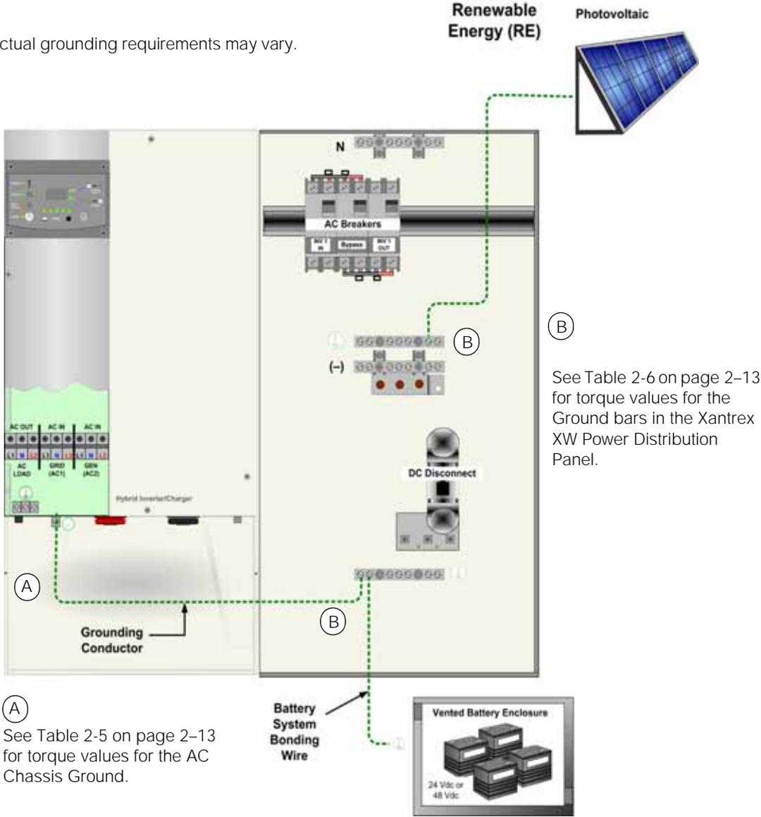
Figure 2-9 DC Grounding Using a Power Distribution Panel
