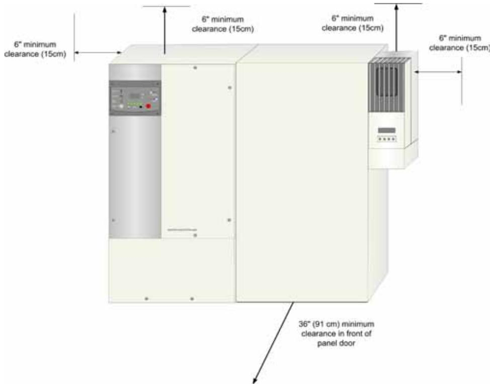
Figure 2-3 Clearance Requirements
