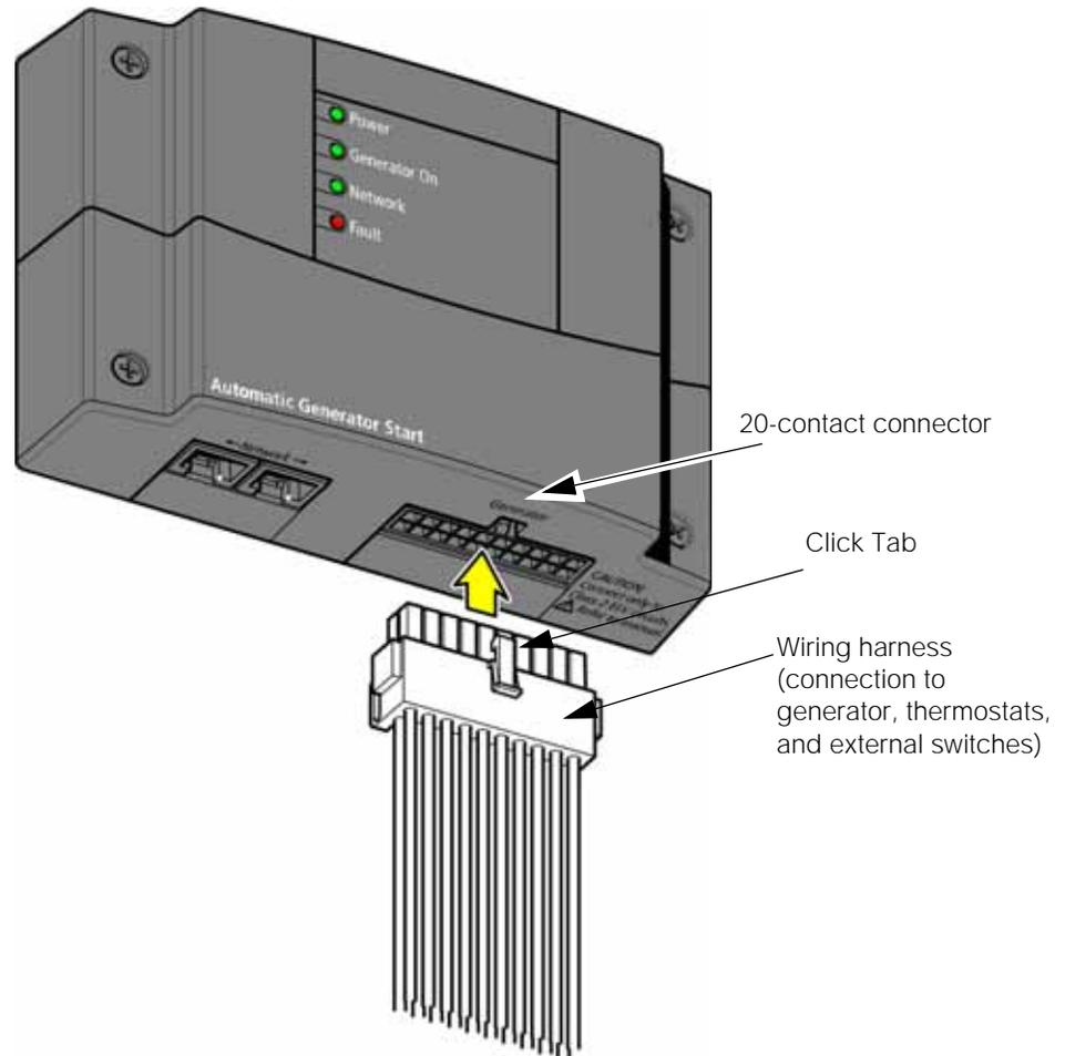
**Figure 5-11** Xantrex XW Automatic Generator Start External Connections
