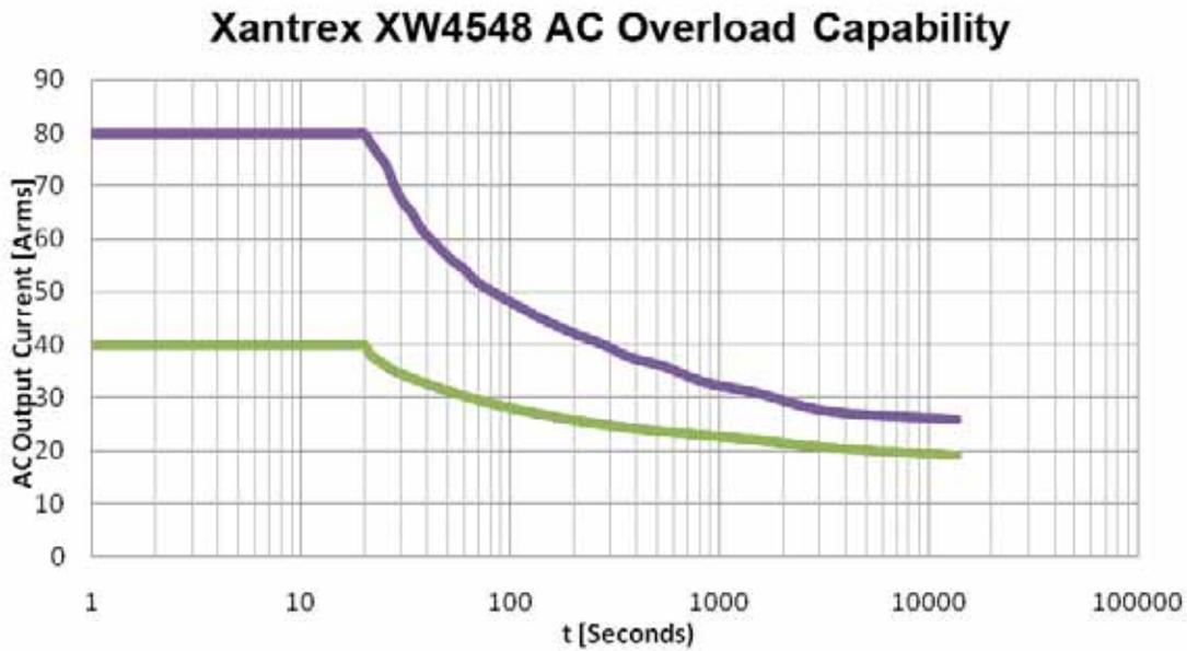
Figure A-2 Xantrex XW Series AC Overload Capability
