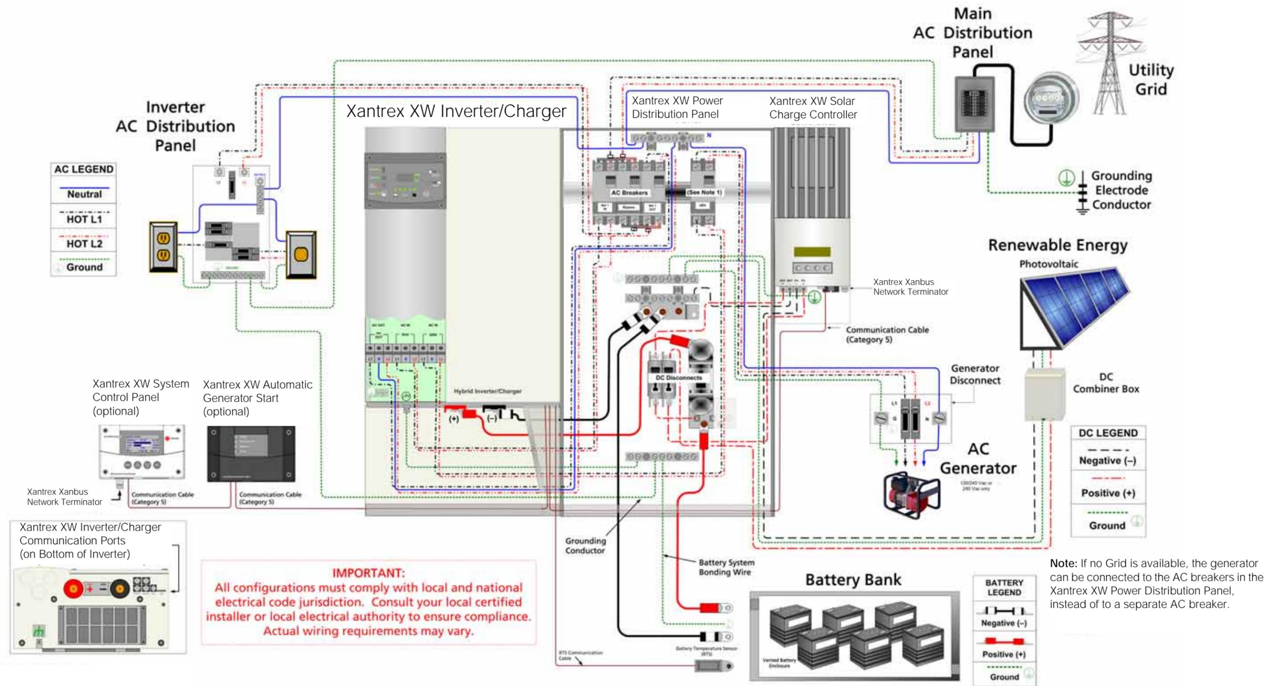
Figure B-3 Single-Inverter System Renewable Energy (Solar)
