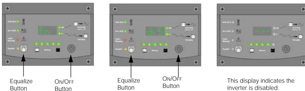
Briefly press the Equalize Button and the ON/OFF Button at the same time to enable or disable the Invert Mode.
