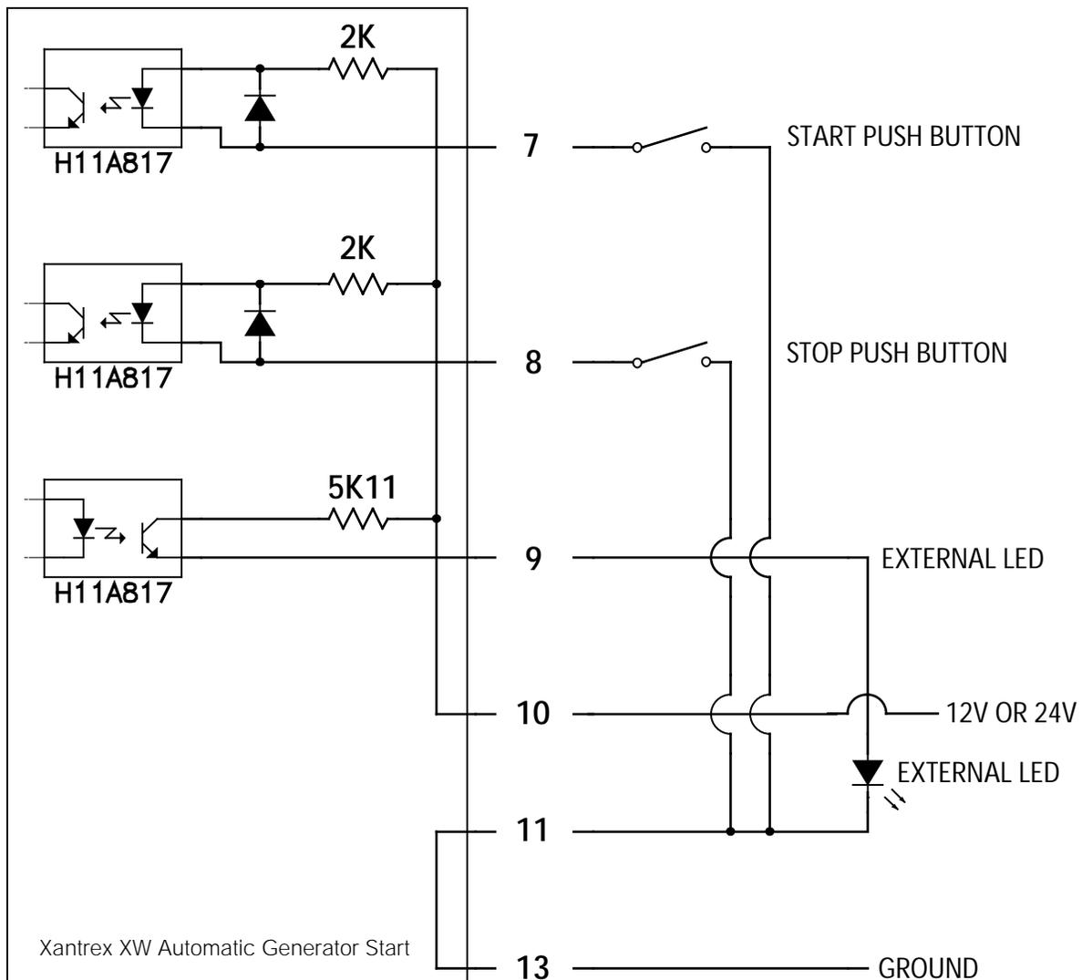
Figure 5-10 External ON/OFF Switch and LED Wiring Diagram
