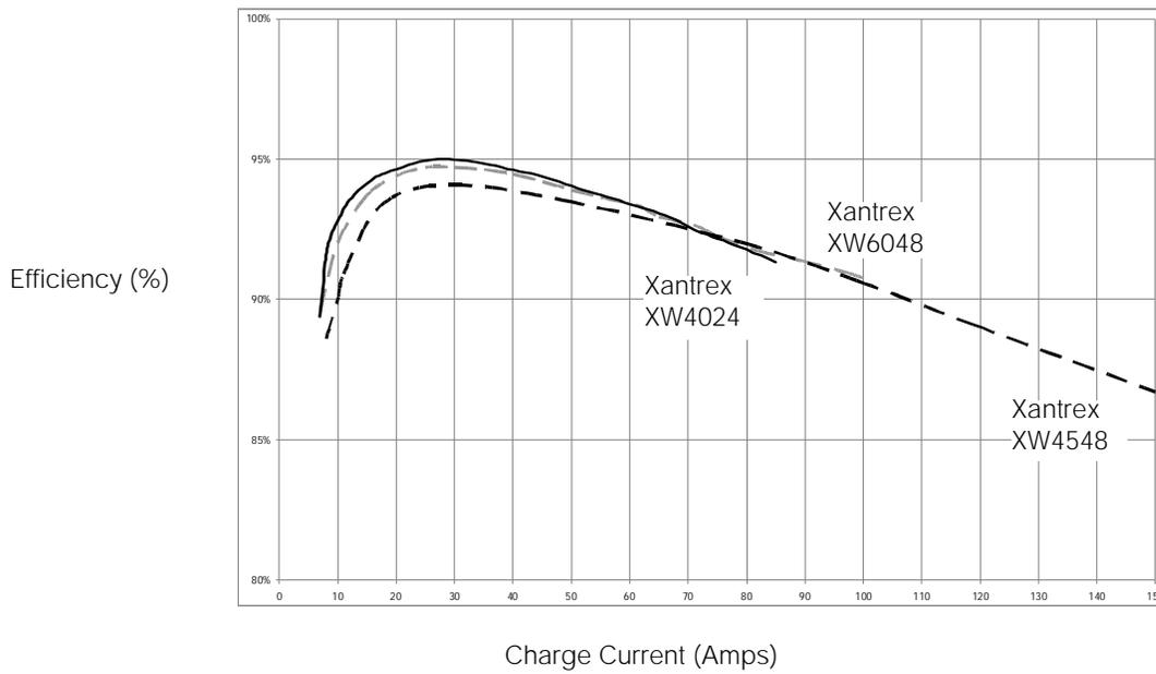
Figure A-6 Charging Efficiency (Typical)
