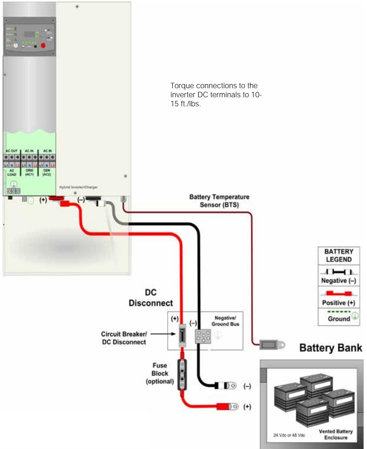
Torque connections to the battery terminals per battery manufacturer's recommendations.
