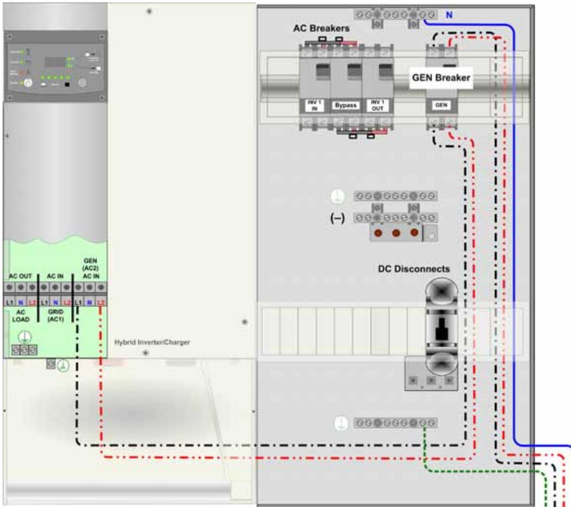
**CAUTION:** Generators must be hard-wired to the Xantrex XW Power Distribution Panel.
