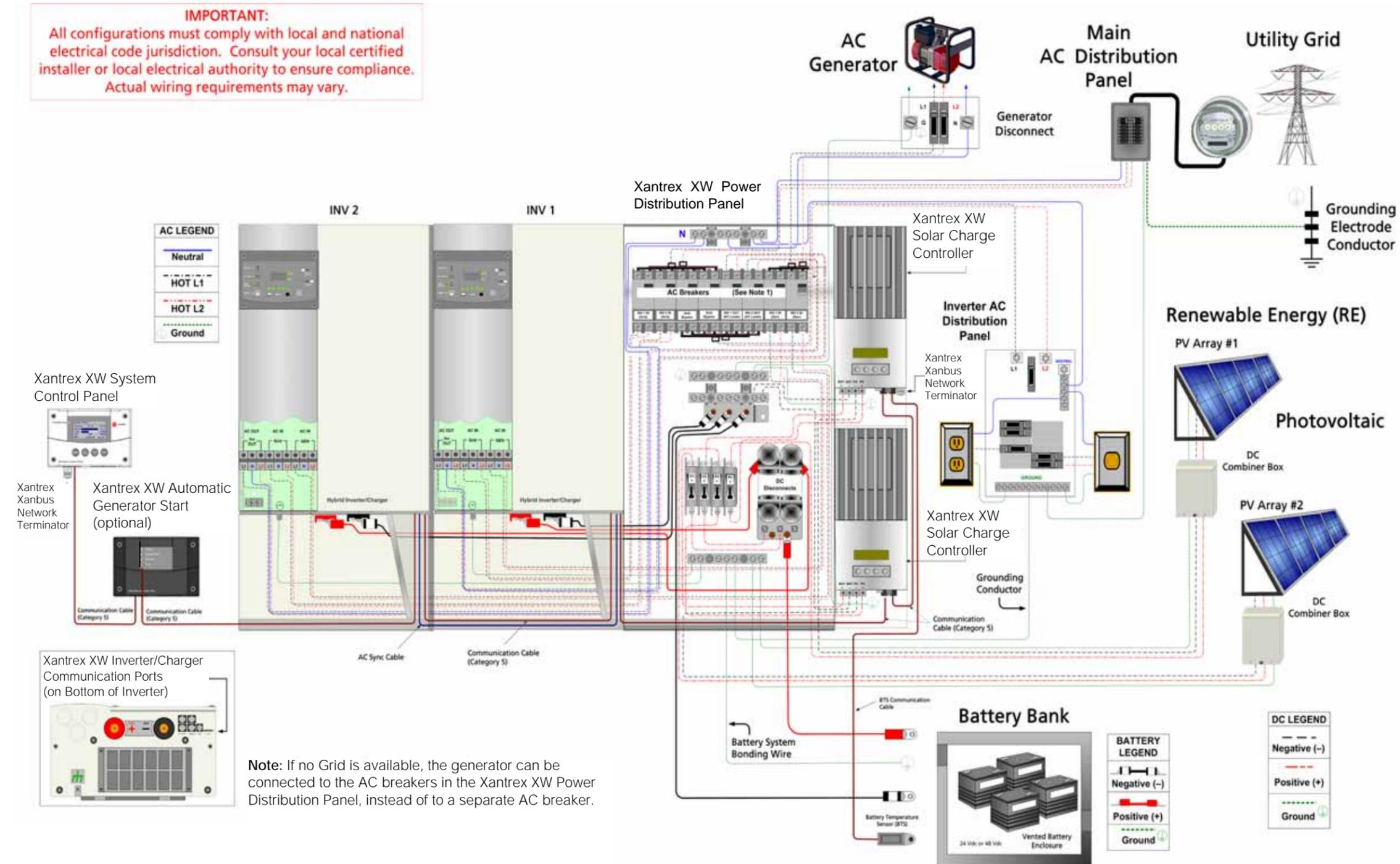
Figure B-5 Dual-Inverter System Renewable Energy (Solar)
