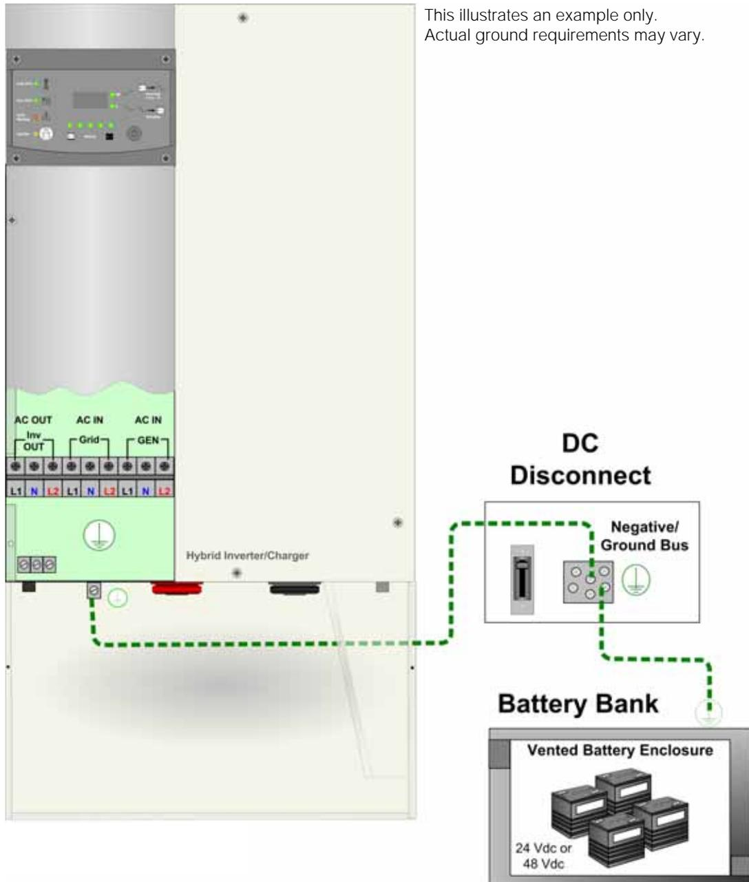
Figure C-1 DC Grounding for an Inverter Only
