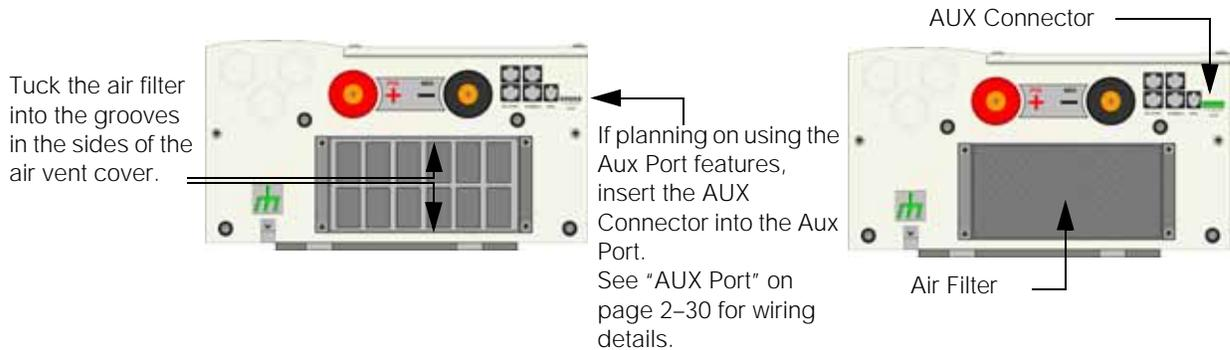
Figure 2-1 Air Filter and AUX Connector Installation
