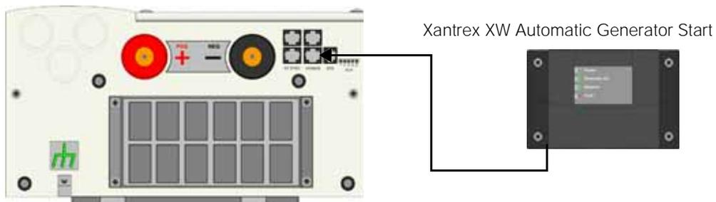
**Figure 5-7** Connecting the Xantrex XW AGS Communications Cable to the Xantrex XW Series
