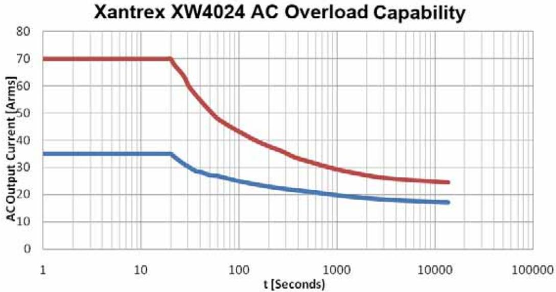
Figure A-3 Xantrex XW Series AC Overload Capability
