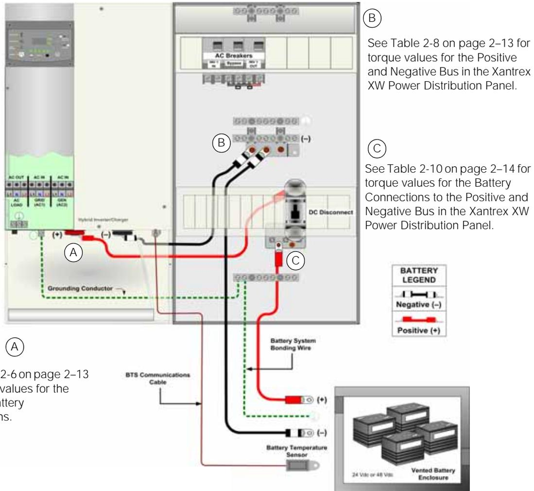
See Table 2-6 on page 2-13 for torque values for the inverter battery connections.
