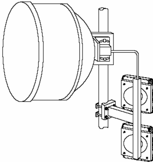
Figure 7-1 Connecting of Single Antenna/Dual ODUs
