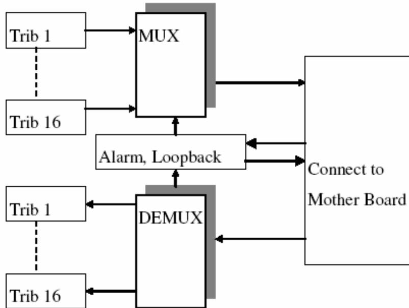
Figure 2-19 Block diagram of the 4/8/16E1 service card
