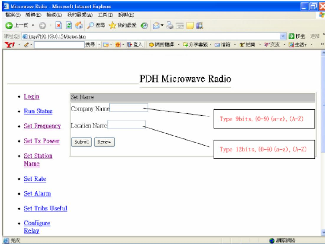
Figure 6-7 Station Name Configuration
