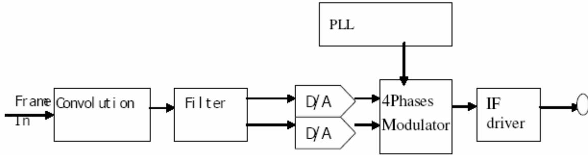
Figure 2-17 Block diagram of the QPSK modulator
