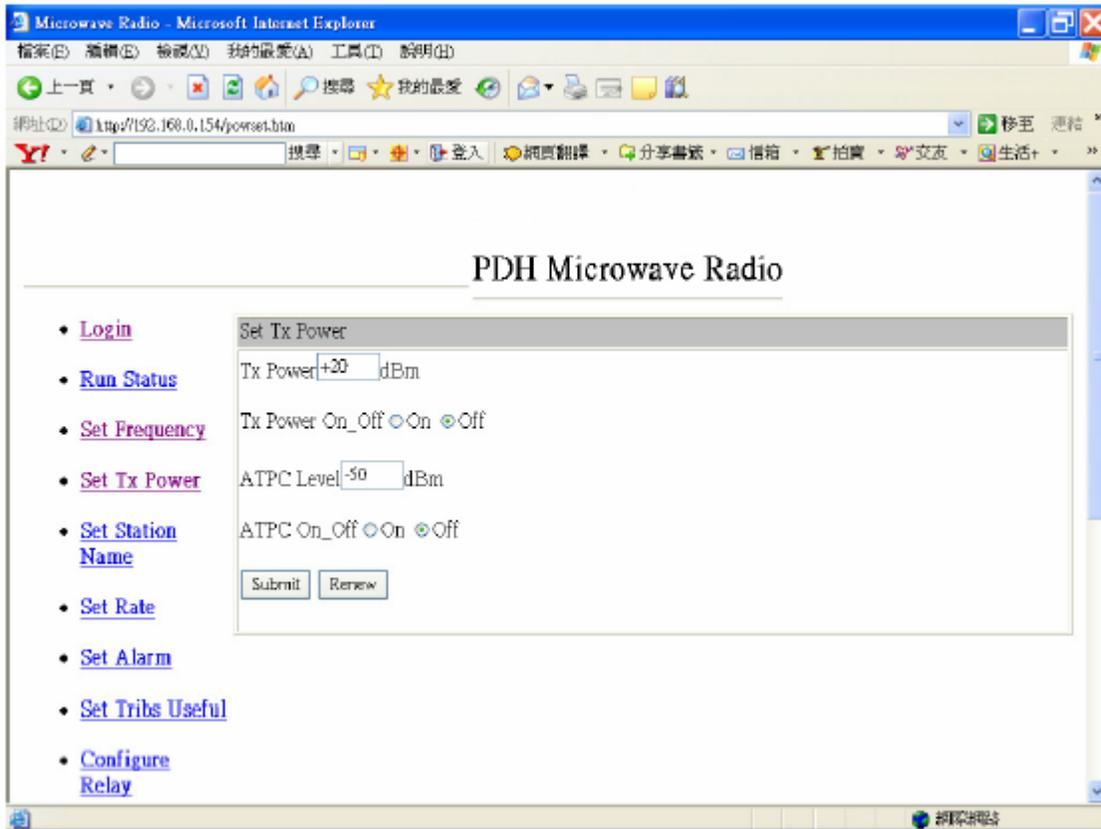
Figure 6-6 Transmit Configuration
