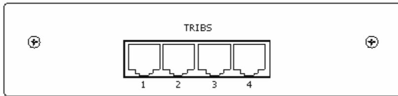
Figure 2-14 4E1 (120ohm balanced) service card
