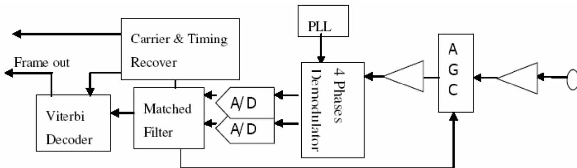
Figure 2-18 Block diagram of the QPSK demodulator
