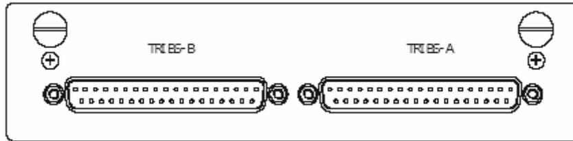
Figure 2-10 4/8/16 E1 (75ohm unbalanced) service card
