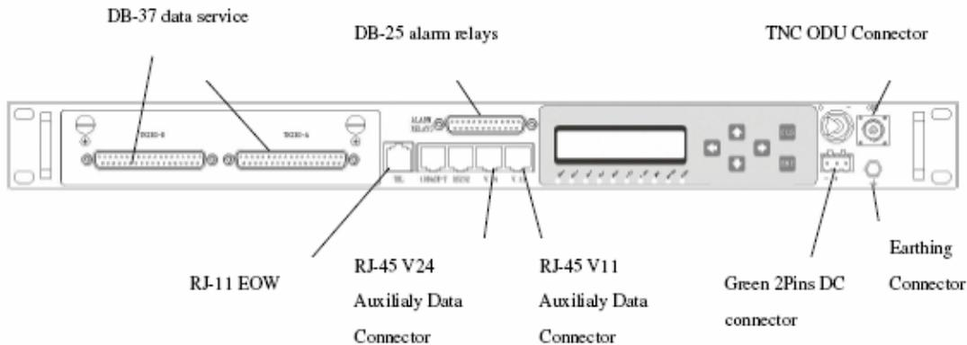
Figure 5-1 Connectors of IDU for 4/8/16E1 75ohm unbalanced Service card
