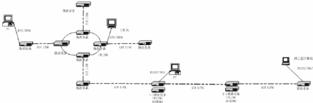
Figure 8-1 Microwave links of Transmission network
