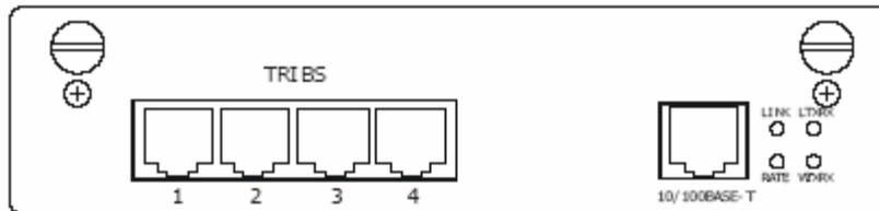
Figure 2-12 10/100BASE-T+1/2/4E1 (120ohm balanced) service card
