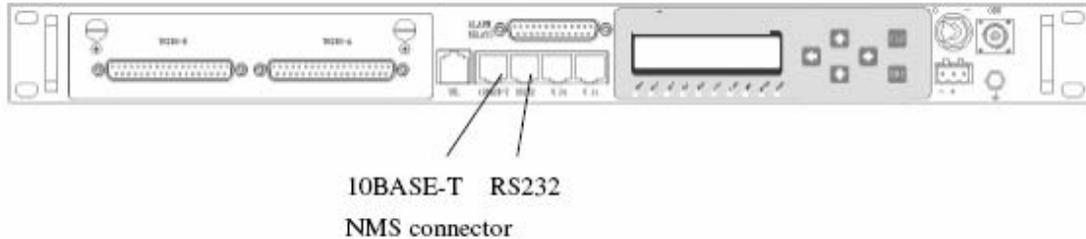
Figure 8-3 NMS connector on IDU
