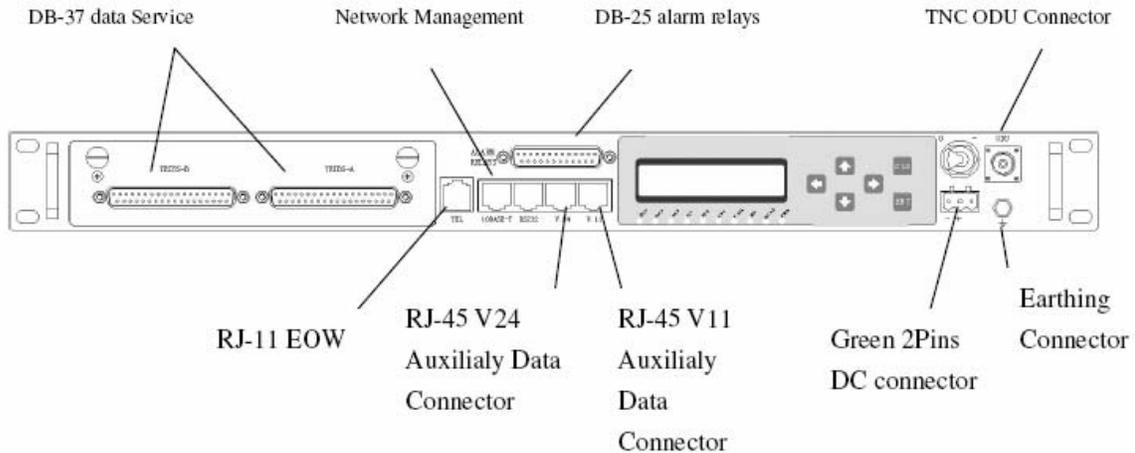
Figure 4-5 Connectors of IDU for 4/8/16E1 75ohm unbalanced Service card
