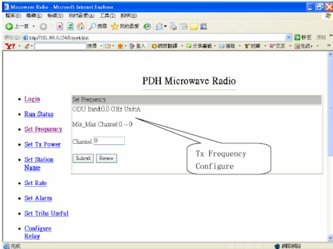
Figure 6-5 Frequency Configuration
