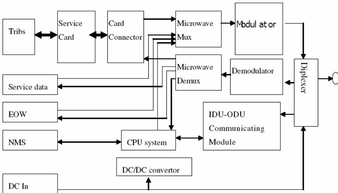
Figure 2-16 Block diagram of the IDU
