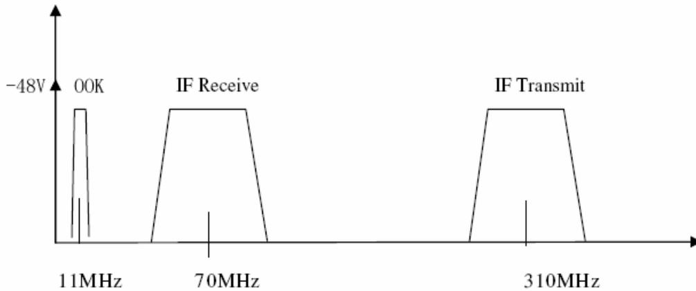
Figure 2-21 Signals in IF Cable
