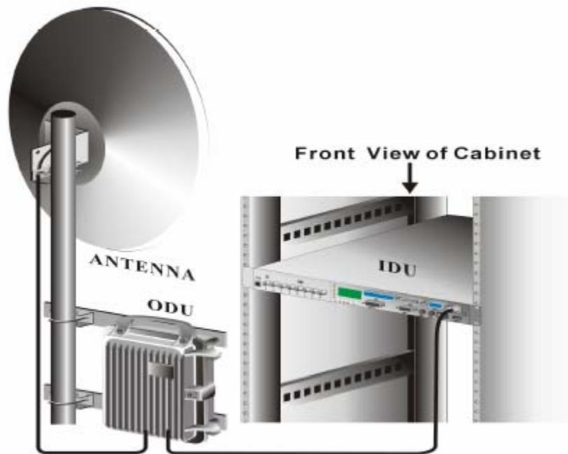
Figure 5-2 Connectnig of Single Antenna
