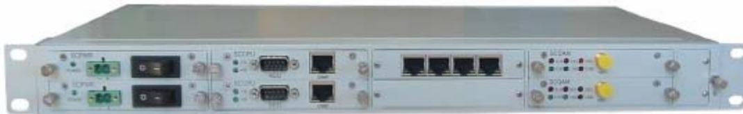
Figure 7-2 IDU protection systems
