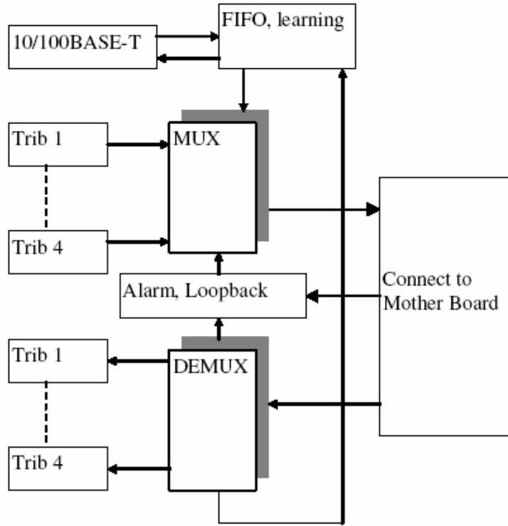
Figure 2-20 Block diagram of the 10/100BASE-T+1/2/4E1 service card
