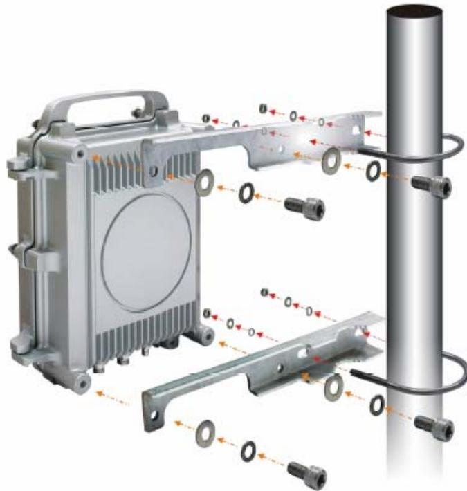
Figure 5-4 Connectors and Mounting of ODU
