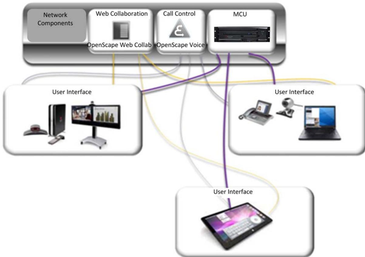
The example configuration shows a Polycom HDX room system in conference with an OpenScope Desktop or Fusion client and a digital device application user. In this case, the video streams are mixed within the Polycom RMX.
