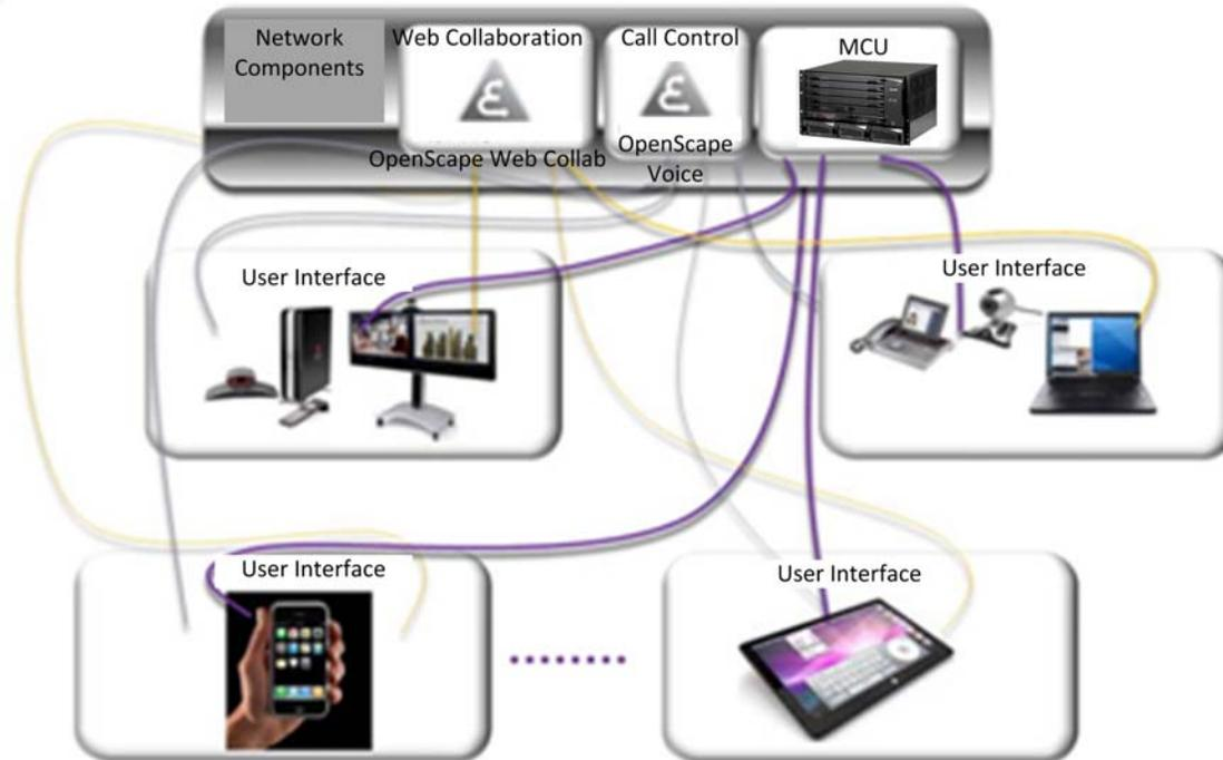
The video conference with a large number of participants in this example is mixed within the Polycom RMX. Collaboration is possible using the OpenScape Web Collaboration application between the room system, OpenScape Desktop Client or Fusion client plus computer, digital device application, and PDA. Plain audio endpoints can also participate in the conference, for example through cell phones or any desk phone.
