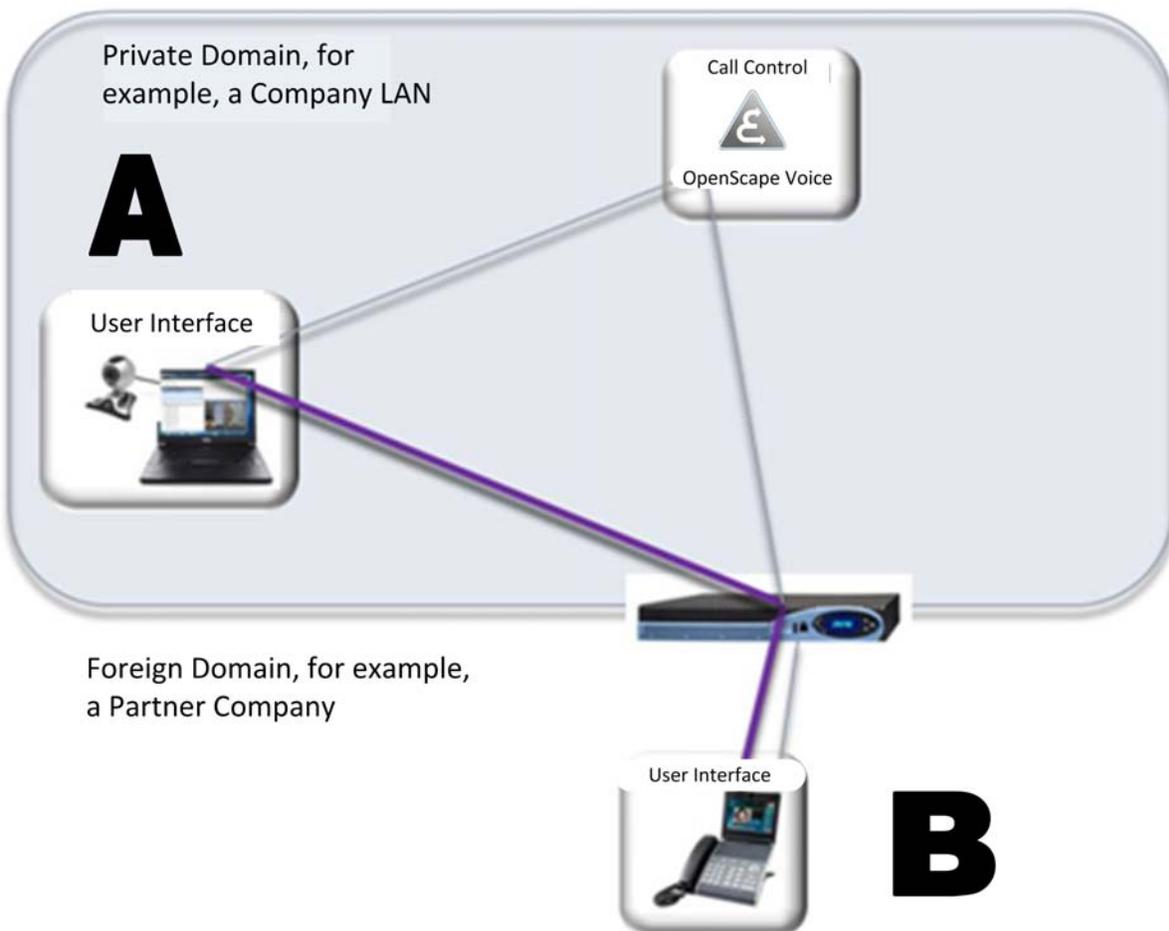
This figure shows a typical video point-to-point call, initiated by an end user in the private domain A, for example, siemens-enterprise.com. It can also be initiated by an endpoint B in a partner company domain, for example, polycom.com.
