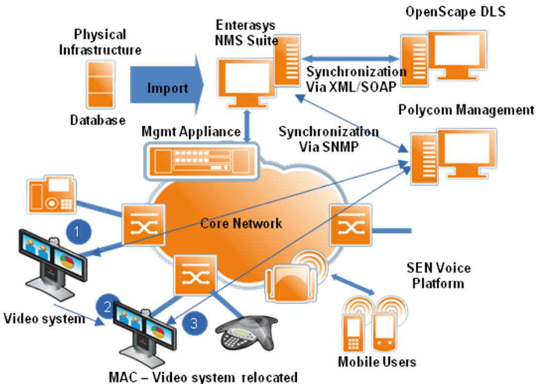
The OpenScope LIA solution provides a constantly updated and automated real-time asset and location service information database for all kinds of end-user systems. This is true even in cases where the end users are new or have moved or been reconfigured.
