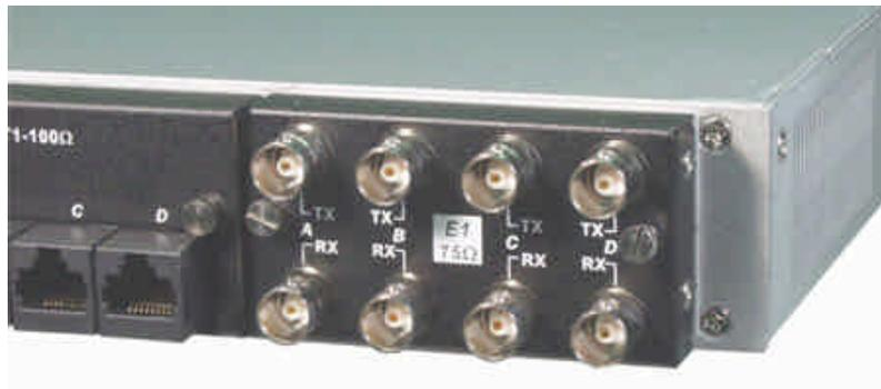
Adapter removed exposing the 4-Channel Port Module
