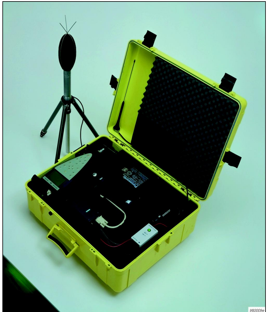
Fig. 5 Field equipment shown with wireless modem. The antenna must be placed to the right in the foam insert, before the lid is closed
