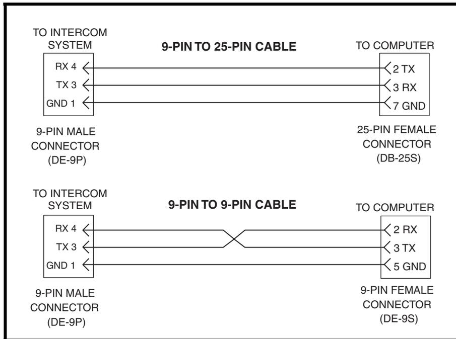
**FIGURE 4.** ADAM CS J900 to Computer Interconnect Cables (ADAM CS with female J900 Connector)
