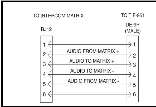
**FIGURE 7.** RJ-11 to 9-pin Intercom Cable. Used for TIF connection to ADAM CS with RJ-11 Back Panel
