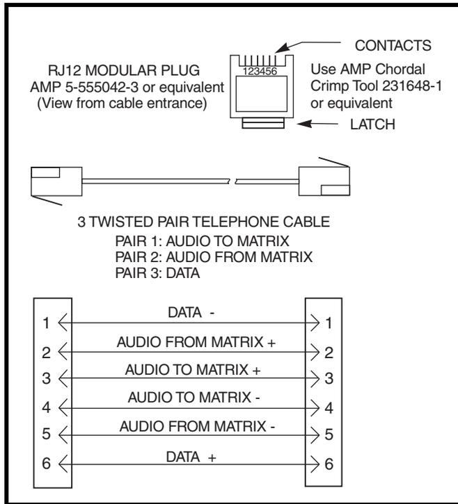
FIGURE 5. RJ-12 Intercom Keypanel Cable
