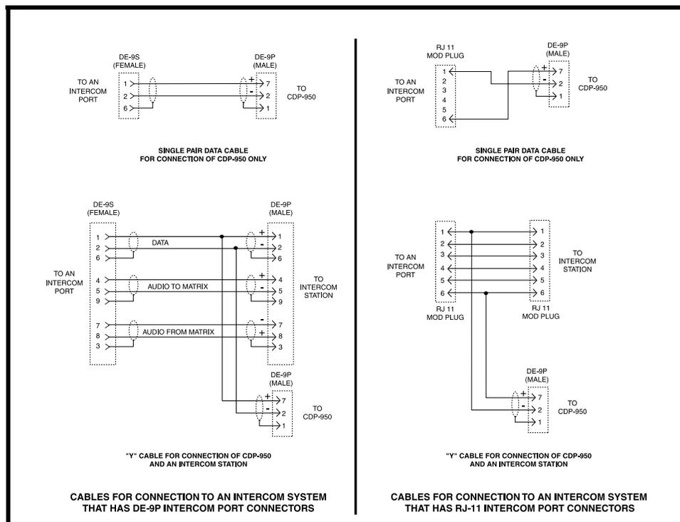
**FIGURE 11.** CDP-950 Cable Wiring Diagrams
