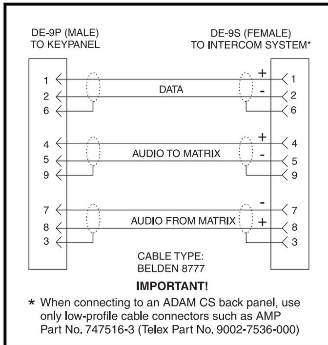
FIGURE 6. 9-pin Intercom Keypanel Cable
