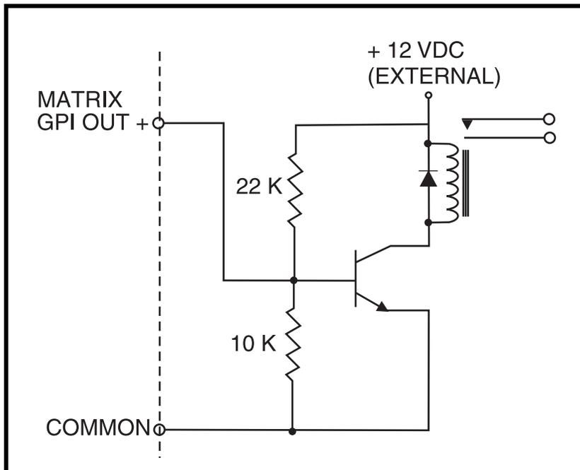
FIGURE 9. Using an ADAM CS GPI Output to Operate a Relay (See Table 1 on page 15 for GPI Connector Pin-out)
