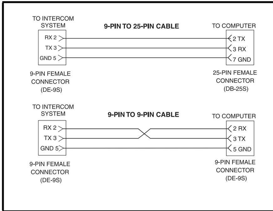
**FIGURE 3.** ADAM CS J900 to Computer Interconnect Cables (ADAM CS with male J900 Connector)
