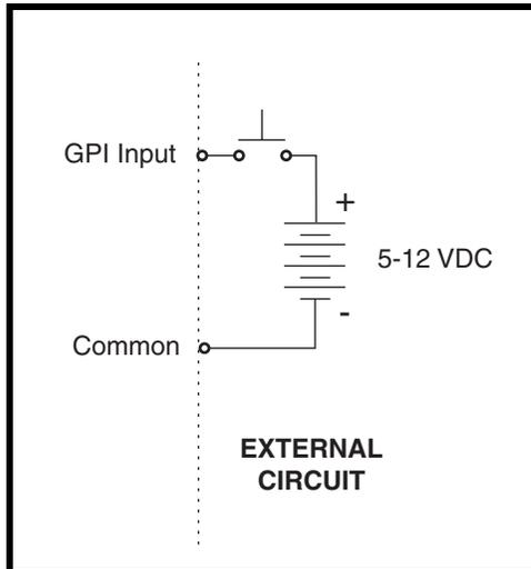
**FIGURE 10.** Using an ADAM GPI Input (See Table 1 on page 15 for GPI Connector Pin-out)
