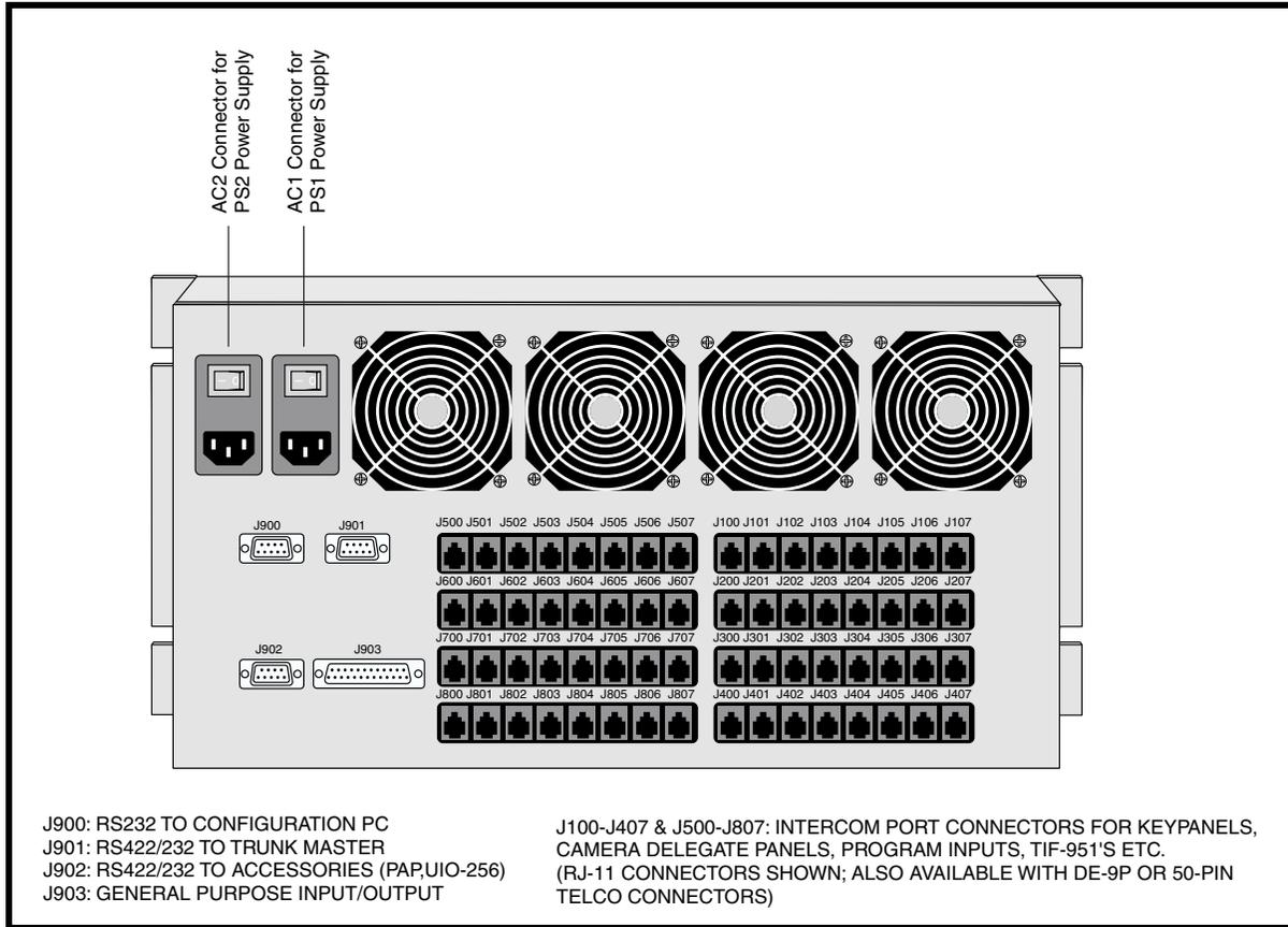
FIGURE 2. ADAM CS Back View (Shown with RJ-11 Connector Panel)
