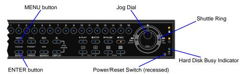
3 To set the Date and Time, press the MENU button. Select Quick Settings, press the ENTER button. Use the shuttle ring to set date and time. Press the MENU button to Exit to the Main Menu.
