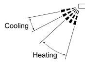
We recommend using the fan in the position listed above when fixing the fan direction.
