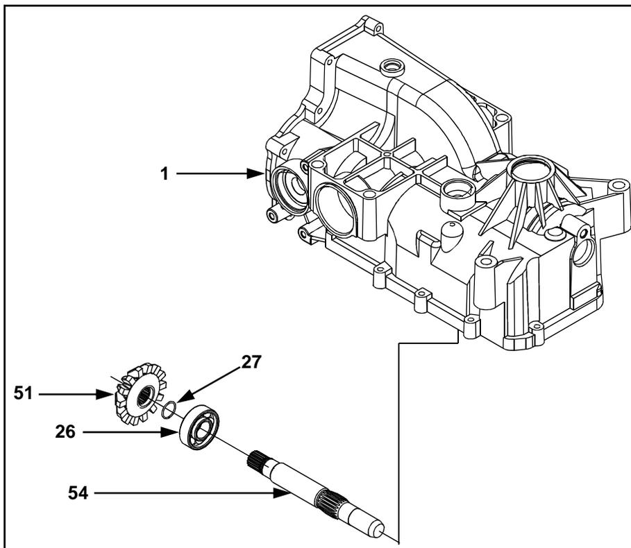
Figure 15. Motor Shaft & Bevel Gear Assembly
