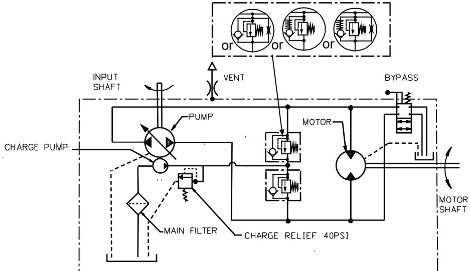
Figure 1. 310-2400/2600 Hydraulic Flow Schematics
