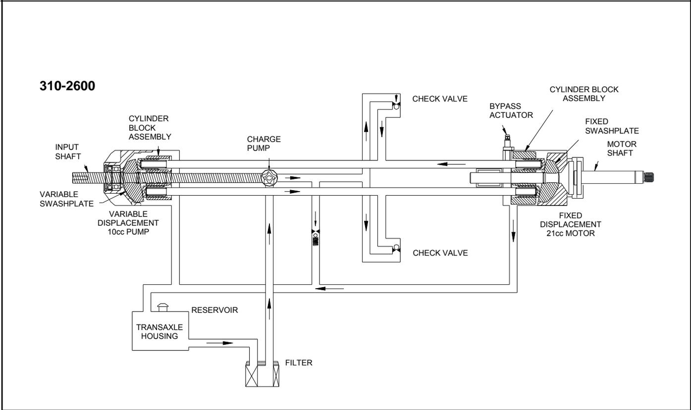
**Figure 2. 310-2400 /2600Hydraulic Flow Illustration**
