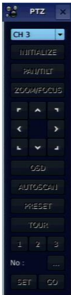
Figure 5.1. PTZ Control Screen
